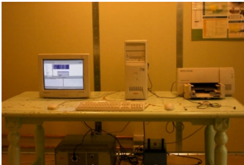
Photograph 2 : Setup for Conducted Emissions
