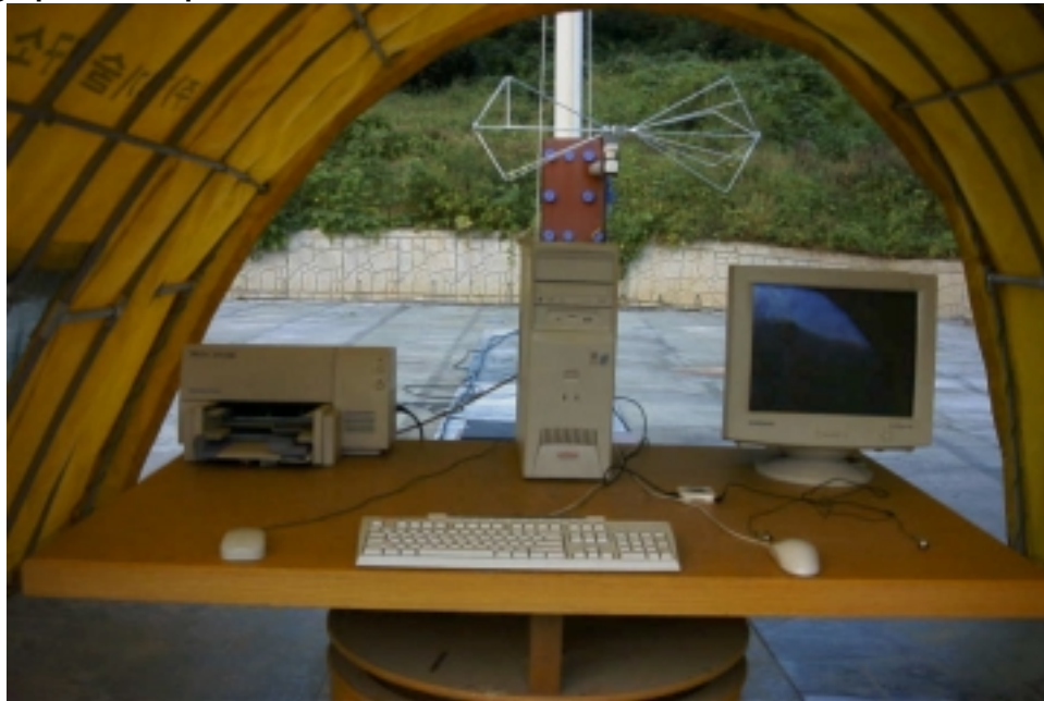
Photograph 1 : Setup for radiated Emissions
