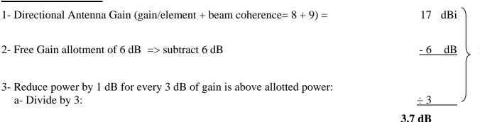
4- The **EMS Tx Power setting** (which is AVE. power/antenna element) = Which is reduced from 1 Watt (30 dBm) limit 4.7 dB > **3.7 dB**.
