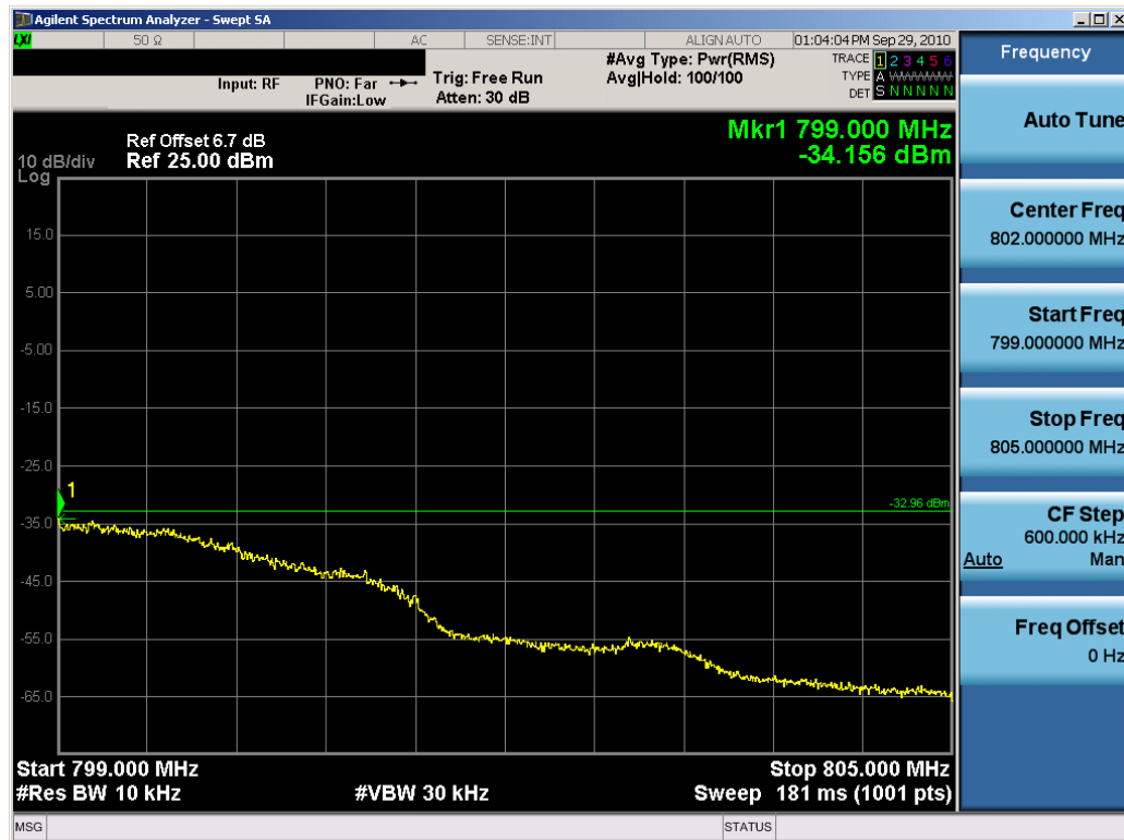
Plot 7-15. Conducted Emissions (799-805MHz) Plot (QPSK)
