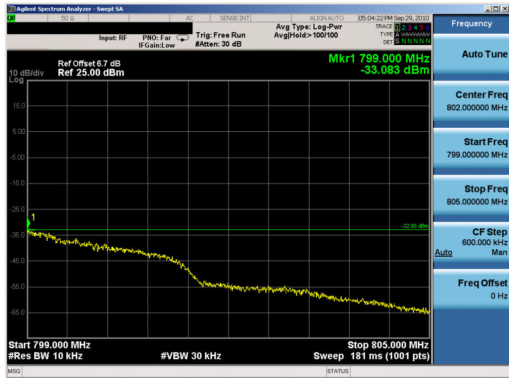
Plot 7-17. Conducted Emissions (799-805MHz) Plot (64QAM)
