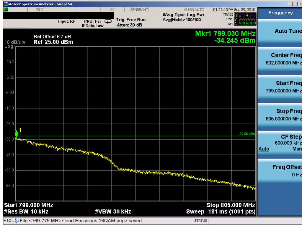
Plot 7-16. Conducted Emissions (799-805MHz) Plot (16QAM)
