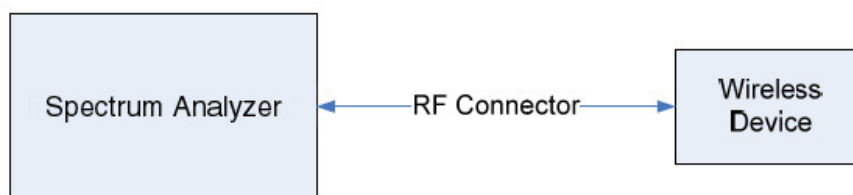
Figure 6-1. Conducted Output Power Test Setup Diagram
