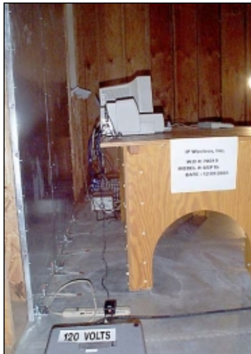
Mains Conducted Emissions Test Setup - Side View
