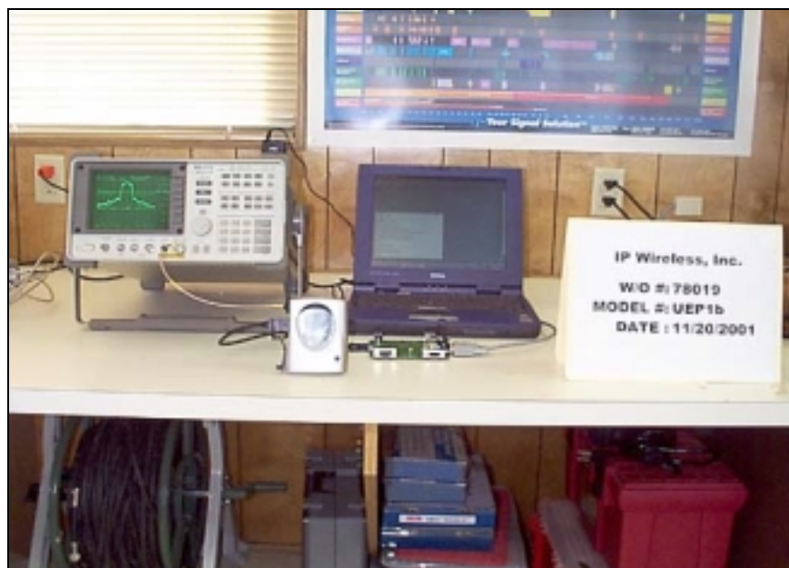
RF Output and Occupied Bandwidth Test Setup
