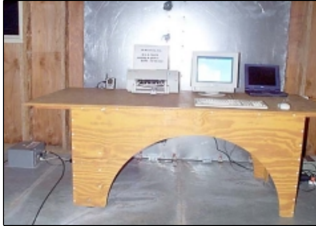
Mains Conducted Emissions Test Setup - Front View
