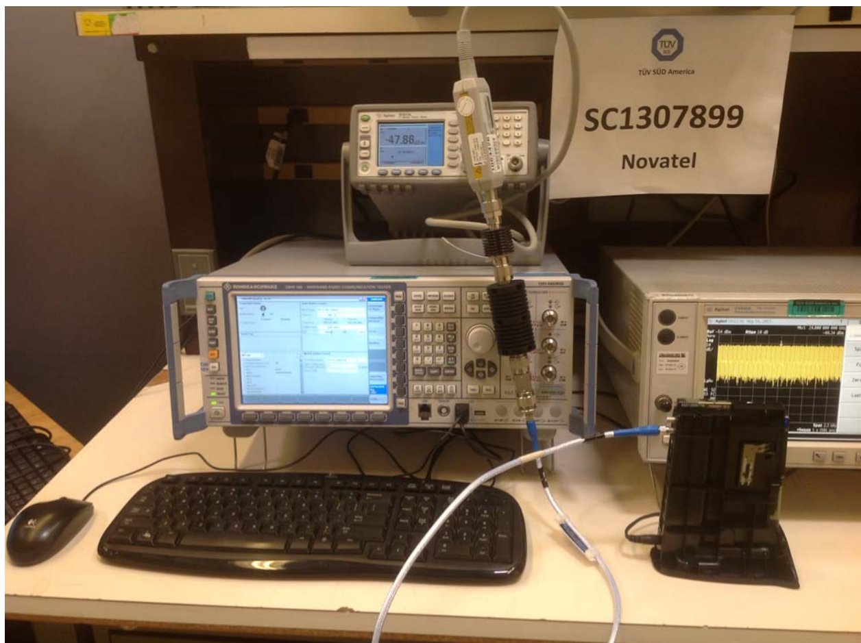
Conducted Port Test Setup 4 (LTE Measurements with Power Analyzer)
