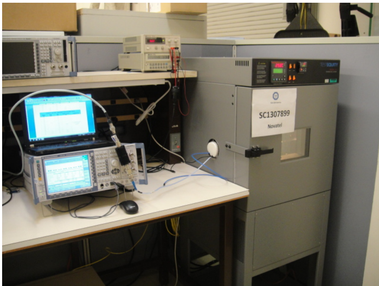
Conducted Port Test Setup 7 (CDMA/LTE Frequency Stability)
