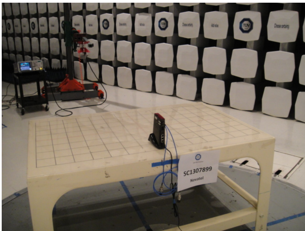
Radiated Emissions Test Setup 2 (WiFi Above 1 GHz)
