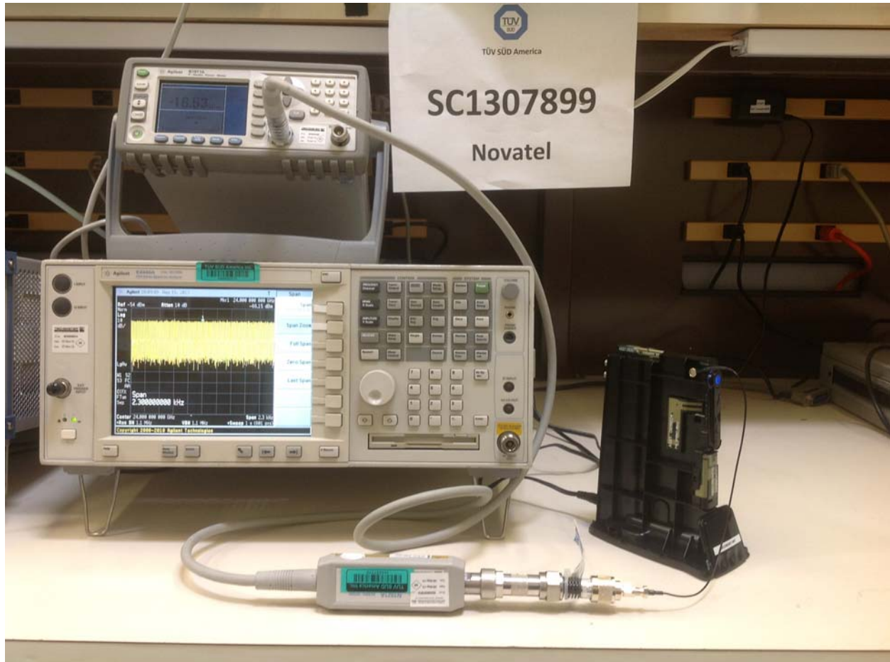
Conducted Port Test Setup 1 (WiFi Max Output power)
