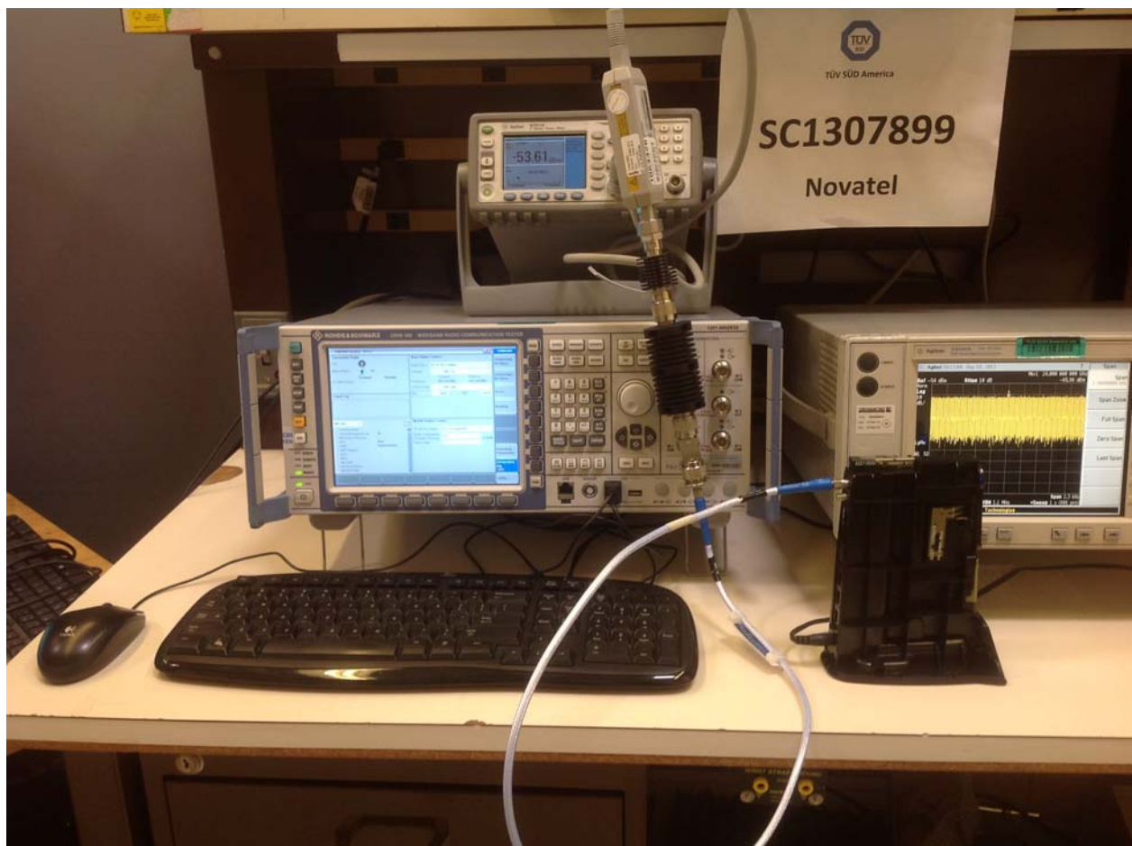
Conducted Port Test Setup 3 (CDMA Measurements with Power Analyzer)
