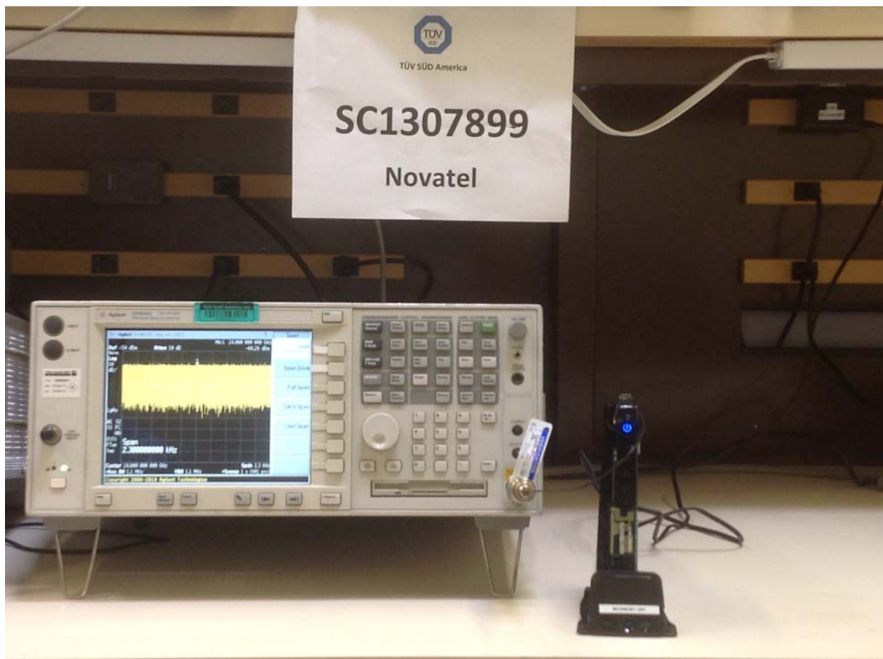
Conducted Port Test Setup 2 (WiFi Measurements with Spectrum Analyzer)
