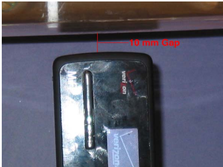
Test Configuration Side C 10 mm Gap
