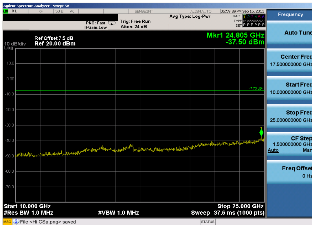
Plot 6-30. Conducted Spurious Plot (802.11b – Ch. 11)
