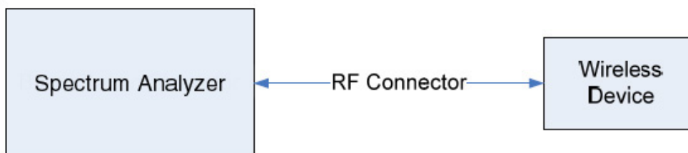
Figure 6-1. WiMAX Conducted Power Test Setup Diagram
