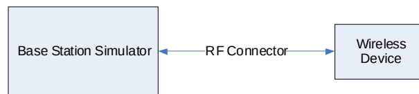
Figure 11-1 Power Measurement Setup
