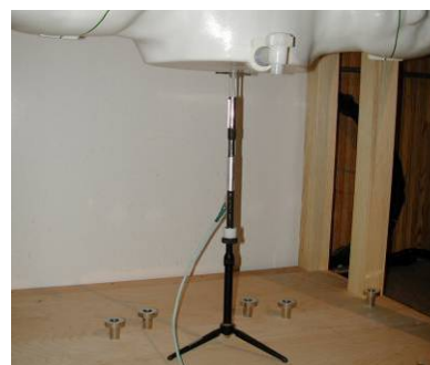
Figure 11-2 System Verification Setup Photo
