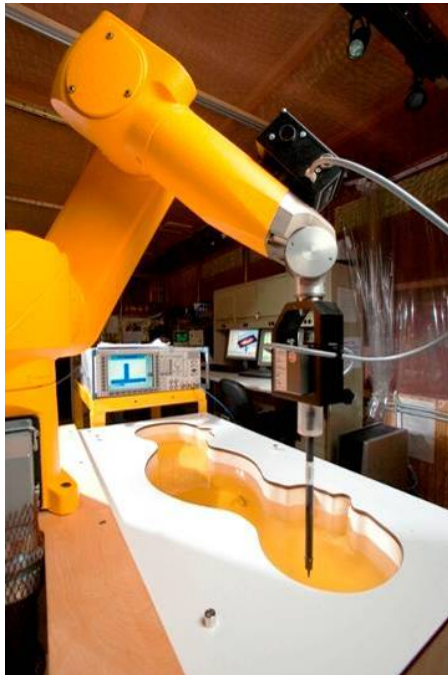
Figure 3-2 SAR Measurement System
