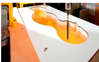
Figure 6-2 SAM Phantom with Simulating Tissue
