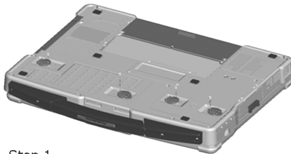
Figure 14-4 Removing a Compartment Door
