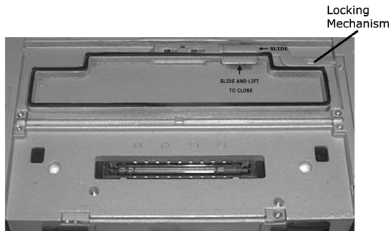
Figure 3-12 XFR630 Docking Device Connector Door in Open/Secured Position
