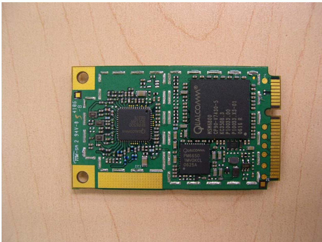
E725 - Bottom side with shields
