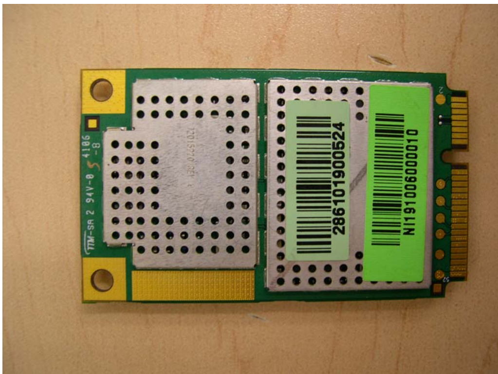
E725 - Bottom side with shields
