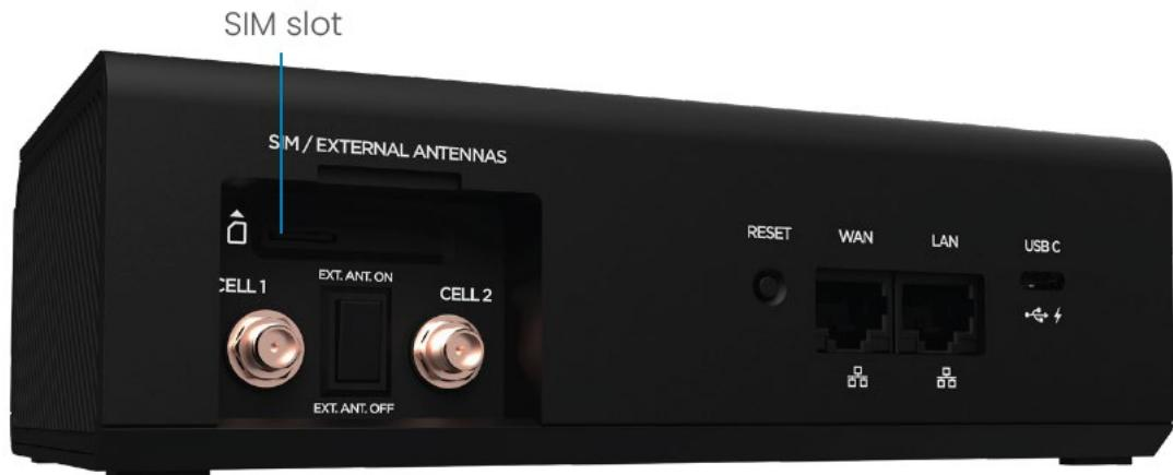
2. If necessary, remove the SIM card from the protective sleeve, being careful not to touch the gold-colored contacts.
