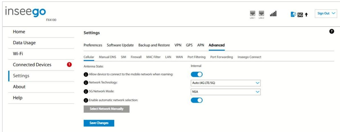
**Antenna State: Internal** indicates the external antenna switch is set to **EXT.ANT.OFF** and all four internal antennas are enabled. **External** indicates the switch is set to **EXT.ANT.ON**.
