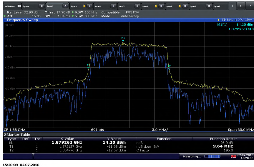
CA_2A-13A_10+10 MHz Bandwidth_PCC_Band 2_1880 MHz_QPSK / 26dB BW
