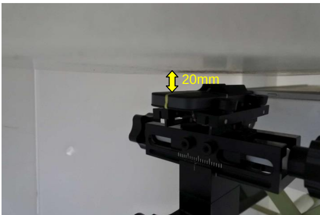
USB Cable Plug-in for USB Configuration 2 (Horizontal Down, Test Separation 20 mm)
