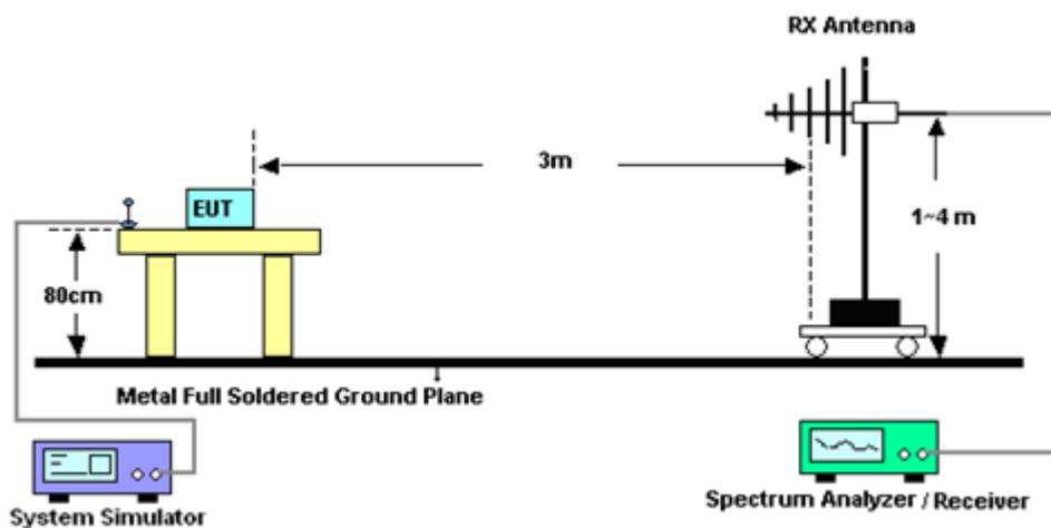
For radiated test from 1GHz to 18GHz
