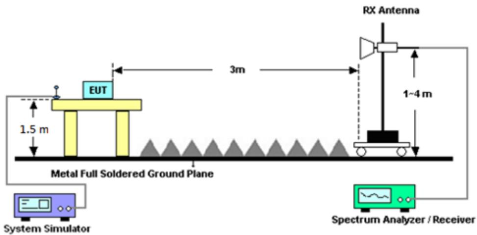
For radiated test above 18GHz
