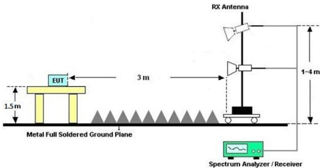
For radiated test above 18GHz
