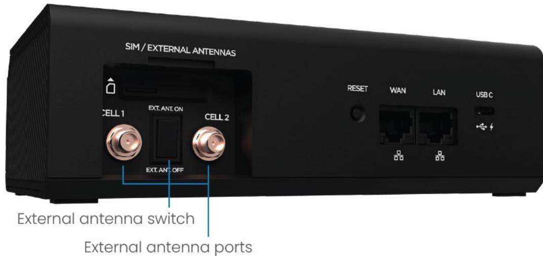
3. Set the switch to **EXT.ANT.ON**. When enabled, each external port supports the full cellular frequency range of 0.6–6 GHz. Two of the internal antennas are disabled. The other two internal antennas remain active. An antenna icon
