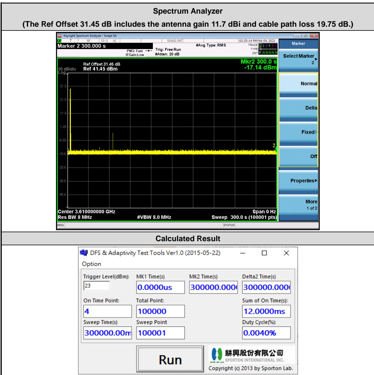
The sum of On Time (aggregated time from marker 1 to 2): 12ms < 10s, Pass.
