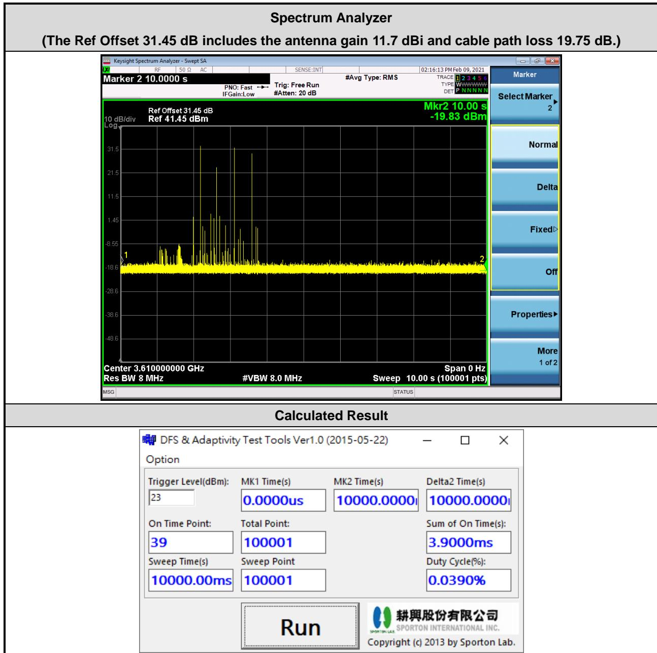
The sum of On Time (aggregated time from marker 1 to 2): 3.9ms < 1s, Pass.
