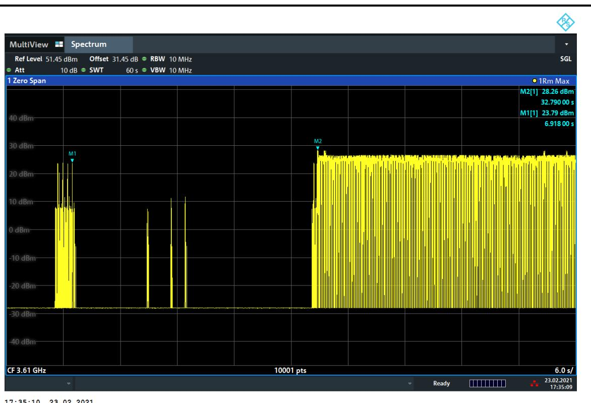
Marker 1: The UUT successfully registered with SAS Test Harness, when operating 23.79 dBm EIRP.
