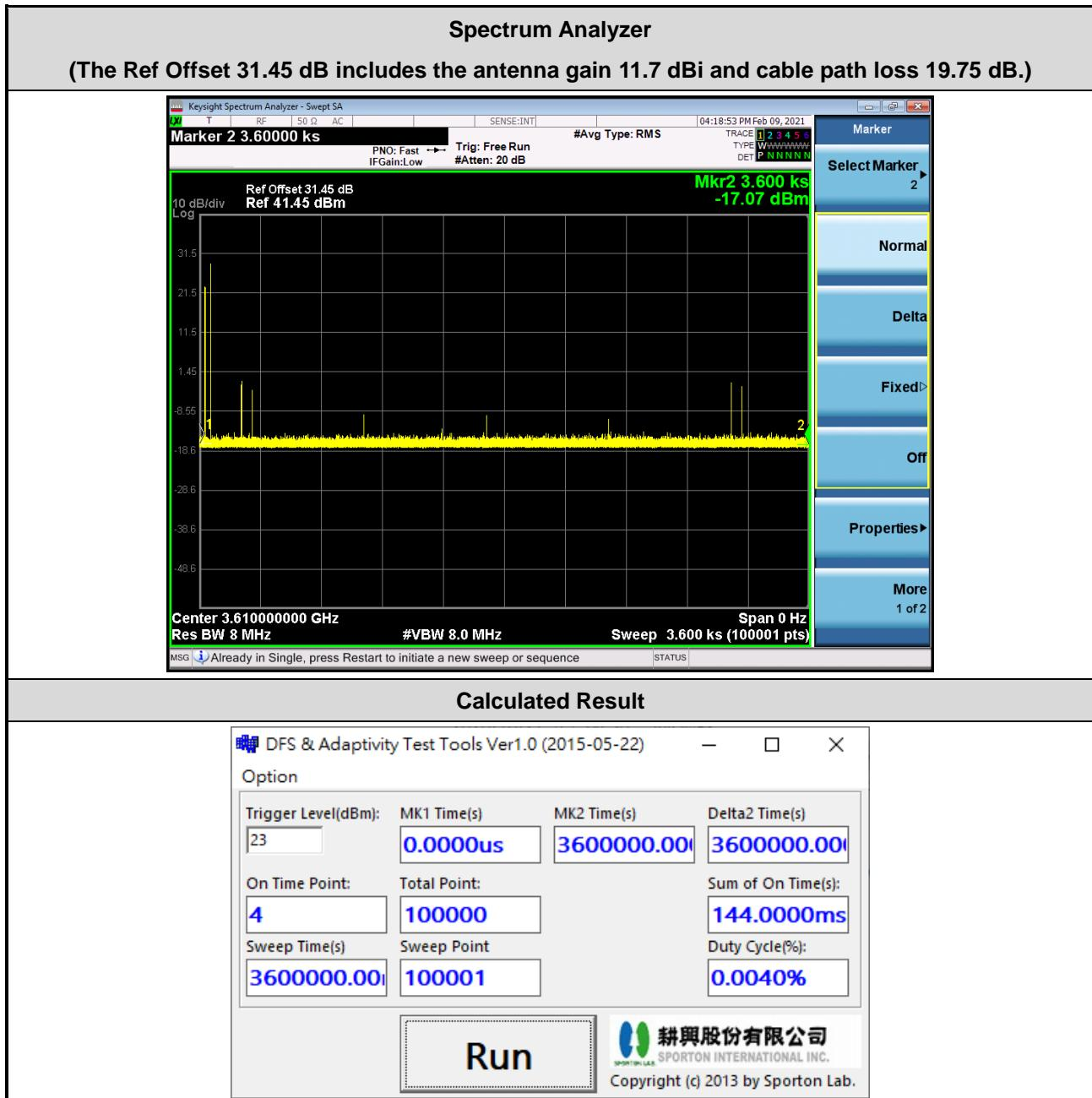
The sum of On Time (aggregated time from marker 1 to 2): 144ms < 20s, Pass.
