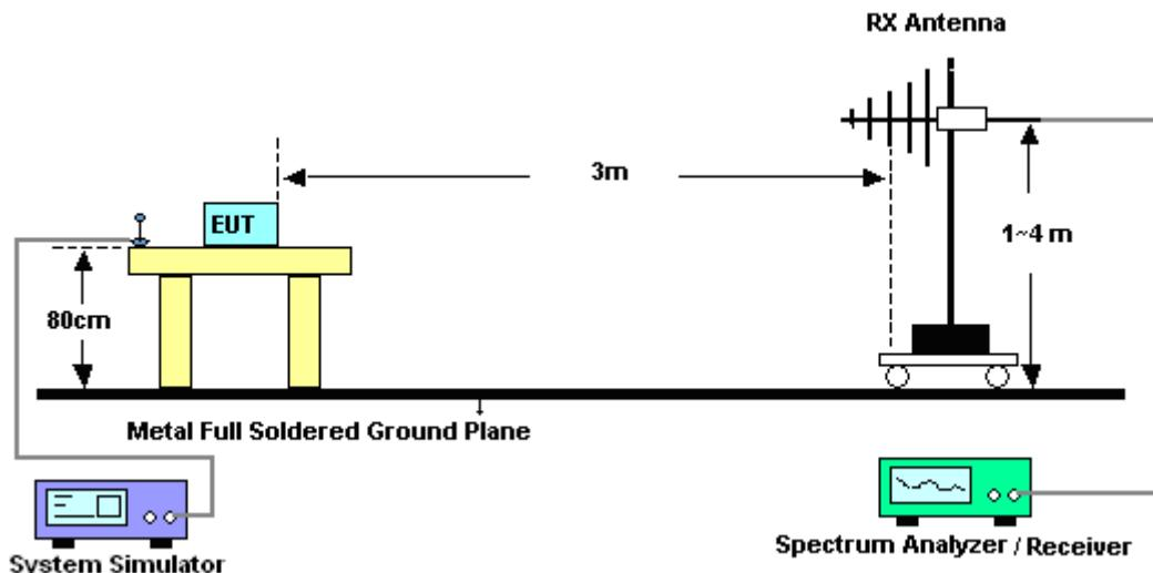
For radiated test above 1GHz
