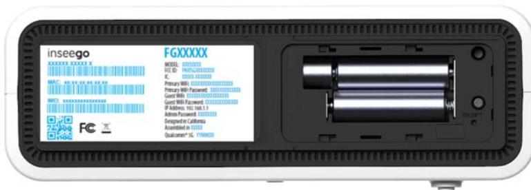
3. Replace the cover by pressing down and sliding it to the right.
