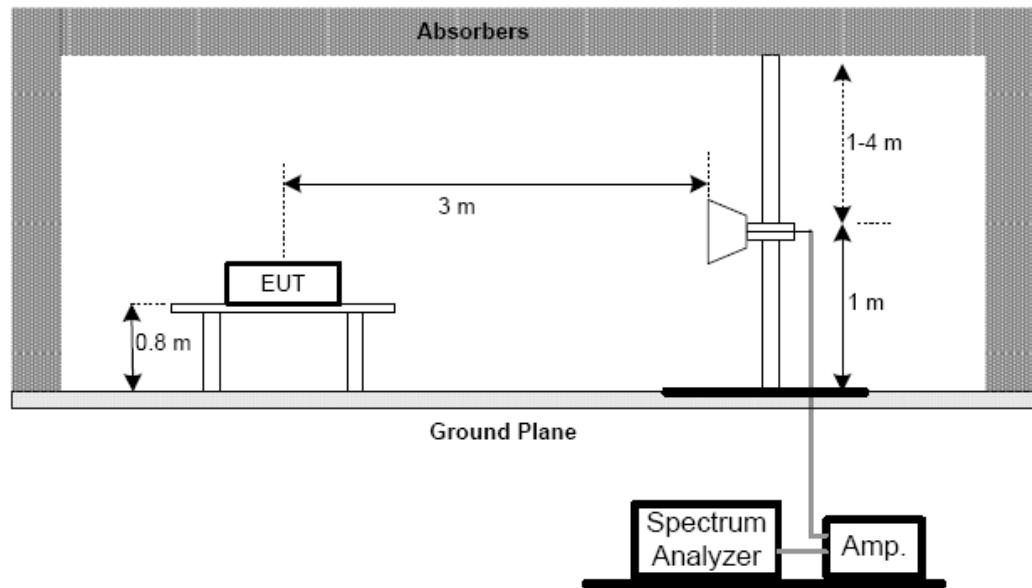
(C) For radiated emissions below 30MHz
