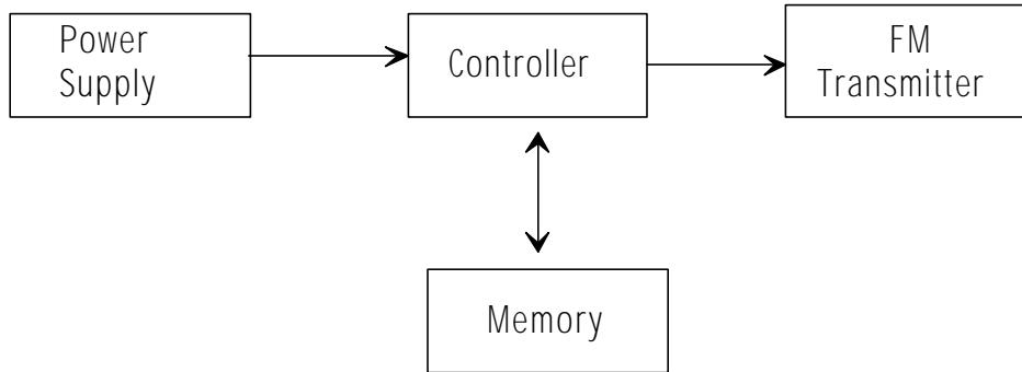
1. The Eseal (433.92MHz) consists of the block as shown above
