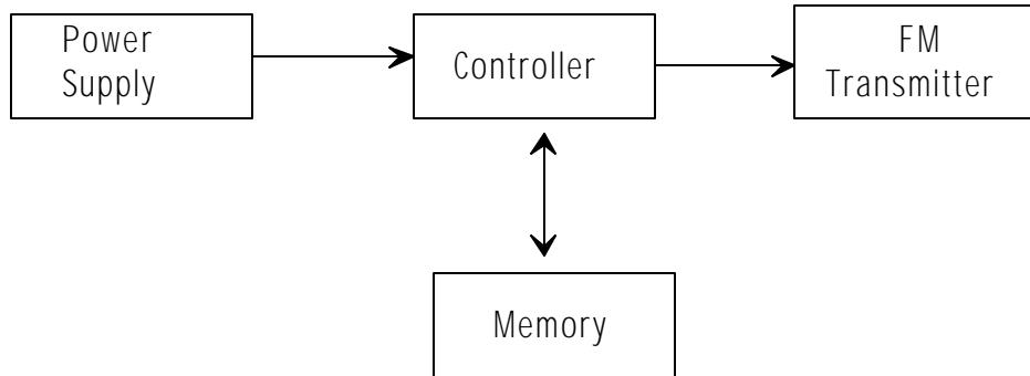
1. The Eseal (315MHz) consists of the block as shown above
