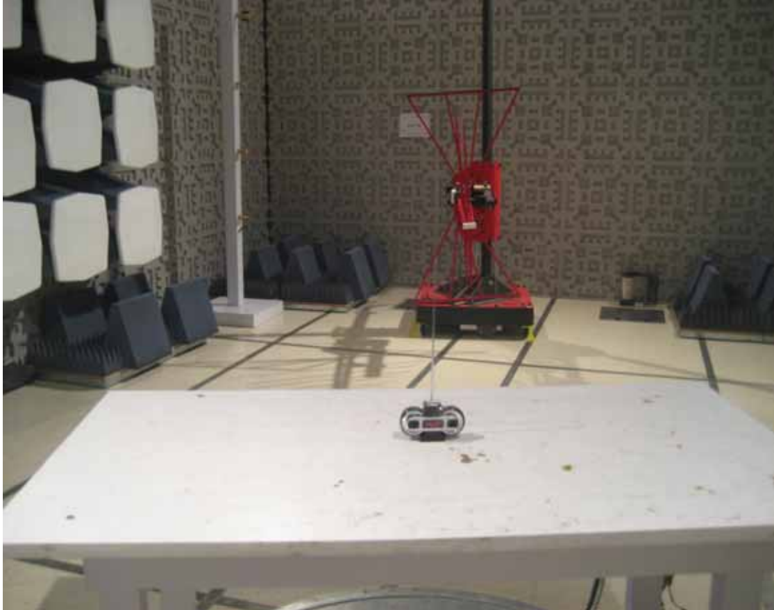
RADIATED EMISSION TEST SETUP
