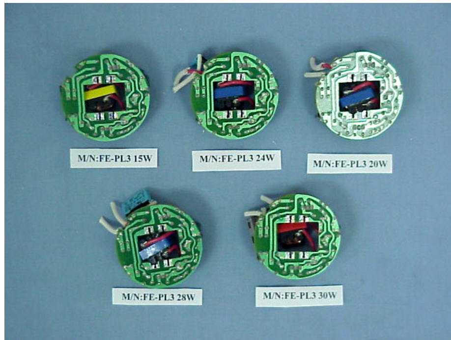
Figure 15. Self-Ballasted Lamp (M/N: FE-PL3 Series) Main Board (Soldered Side)
