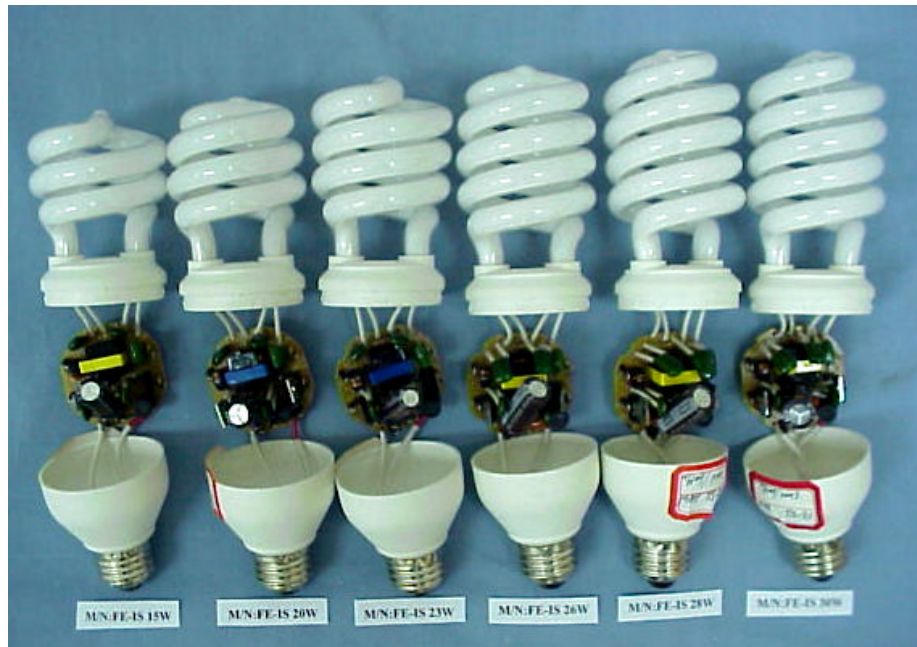
Figure 7. Self-Ballasted Lamp (M/N: FE-IS Series) Cover Removed
