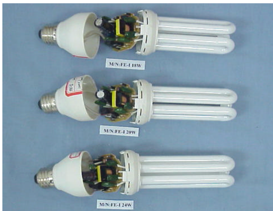
Figure 1. Self-Ballasted Lamp (M/N: FE-I Series) Cover Removed
