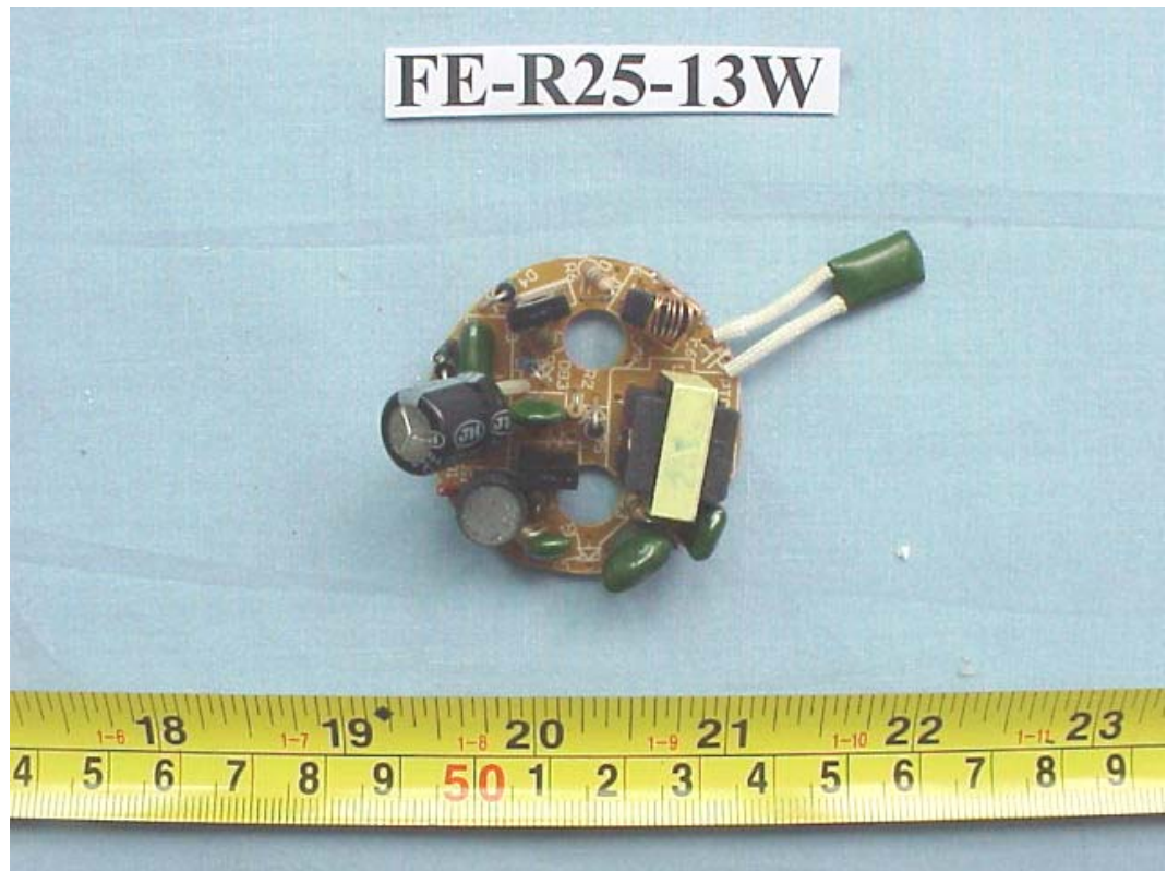
FIGURE 7 ENERGY SAVING LAMP (M/N: FE-R25-13W) MAIN BOARD (COMPONENT SIDE)
