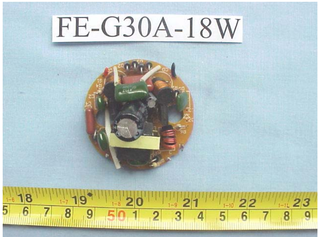
FIGURE 31 ENERGY SAVING LAMP (M/N: FE-G30A-18W) MAIN BOARD (COMPONENT SIDE)
