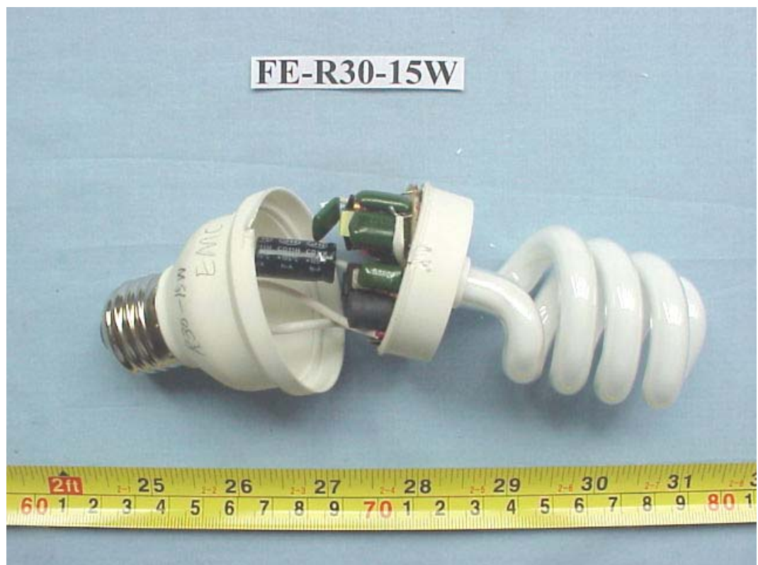
FIGURE 10 ENERGY SAVING LAMP (M/N: FE-R30-15W) COVER REMOVED 2
