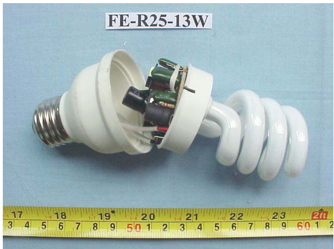
FIGURE 6 ENERGY SAVING LAMP (M/N: FE-R25-13W) COVER REMOVED 2
