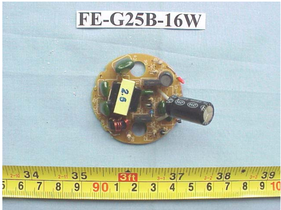
FIGURE 27 ENERGY SAVING LAMP (M/N: FE-G25B-16W) MAIN BOARD (COMPONENT SIDE)
