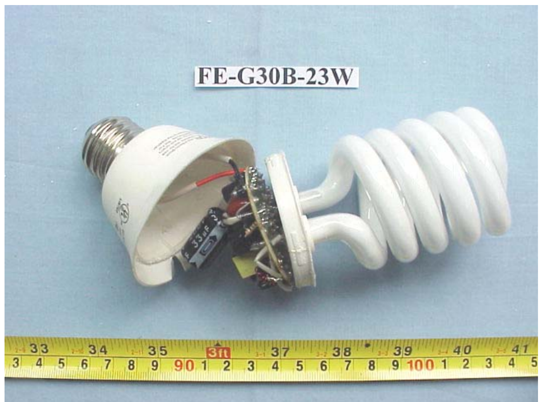
FIGURE 34 ENERGY SAVING LAMP (M/N: FE-G30B-23W) COVER REMOVED 2
