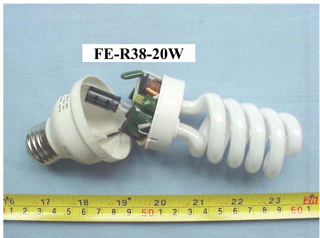
FIGURE 14 ENERGY SAVING LAMP (M/N: FE-R38-20W) COVER REMOVED 2
