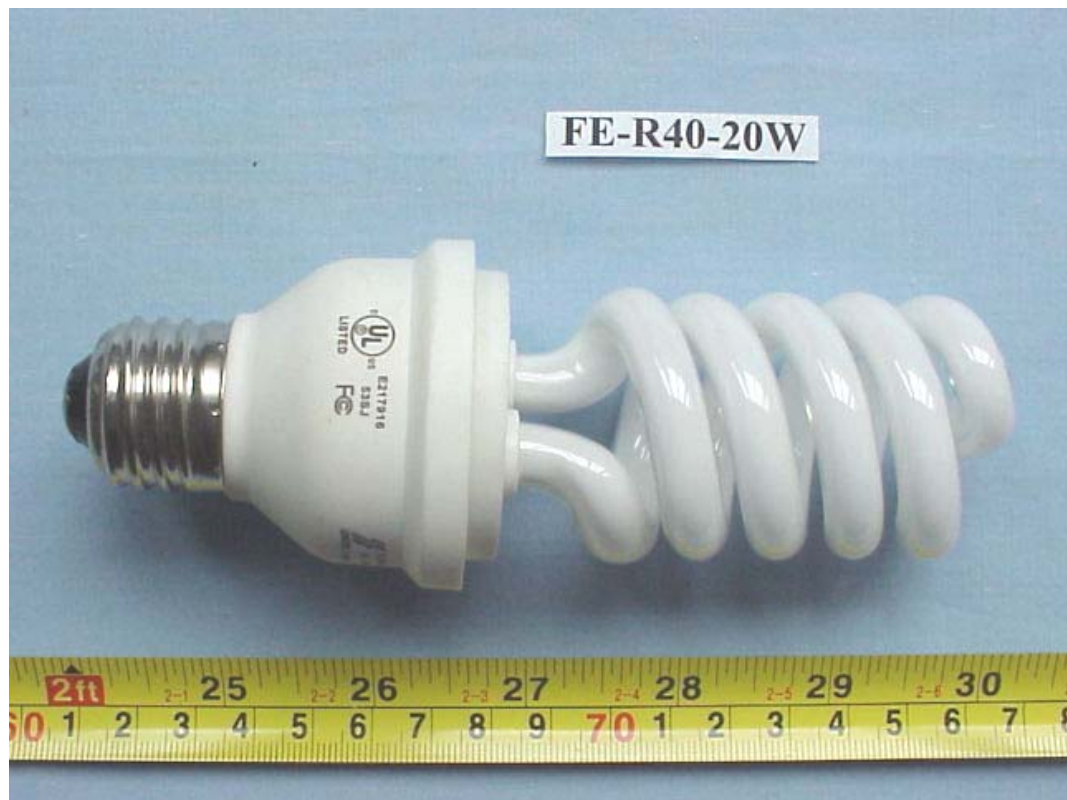
FIGURE 17 ENERGY SAVING LAMP (M/N: FE-R40-20W) COVER REMOVED 1
