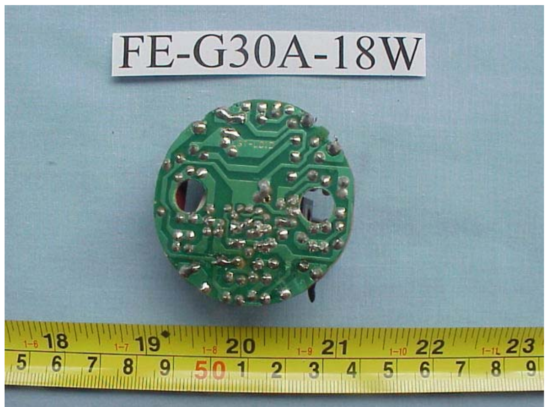
FIGURE 32 ENERGY SAVING LAMP (M/N: FE-G30A-18W) MAIN BOARD (SOLDERED SIDE)
