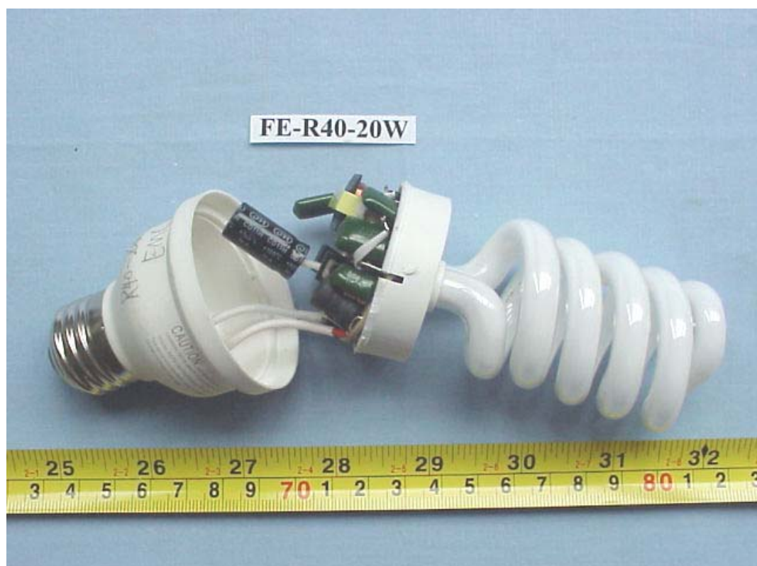
FIGURE 18 ENERGY SAVING LAMP (M/N: FE-R40-20W) COVER REMOVED 2
