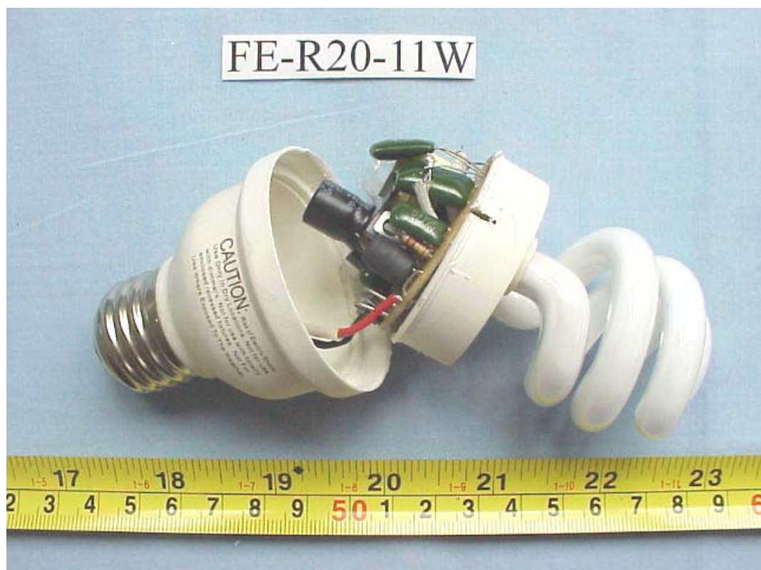
FIGURE 2 ENERGY SAVING LAMP (M/N: FE-R20-11W) COVER REMOVED 2
