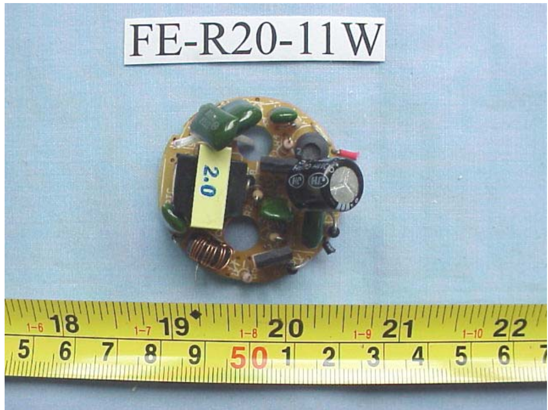
FIGURE 3 ENERGY SAVING LAMP (M/N: FE-R20-11W) MAIN BOARD (COMPONENT SIDE)
