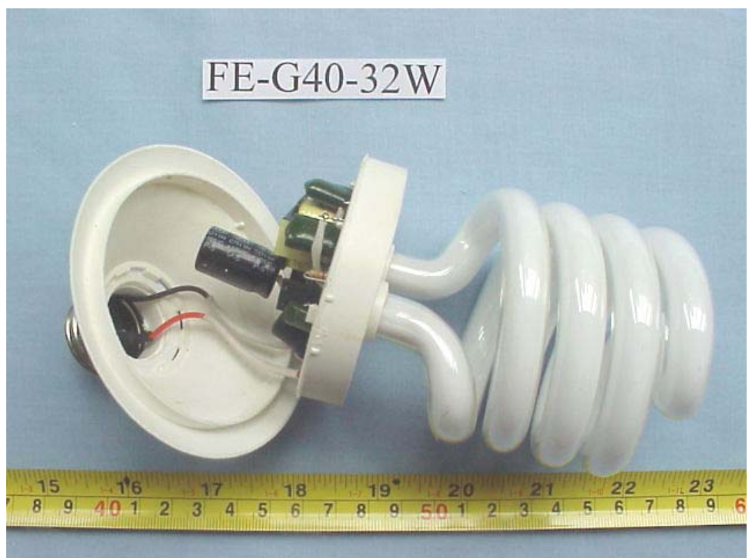
FIGURE 38 ENERGY SAVING LAMP (M/N: FE-G40-32W) COVER REMOVED 2
