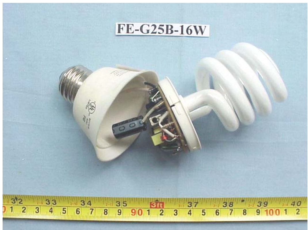
FIGURE 26 ENERGY SAVING LAMP (M/N: FE-G25B-16W) COVER REMOVED 2
