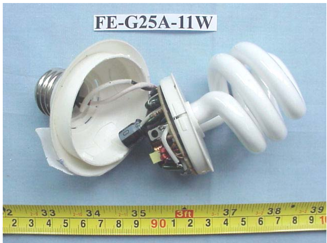
FIGURE 22 ENERGY SAVING LAMP (M/N: FE-G25A-11W) COVER REMOVED 2
