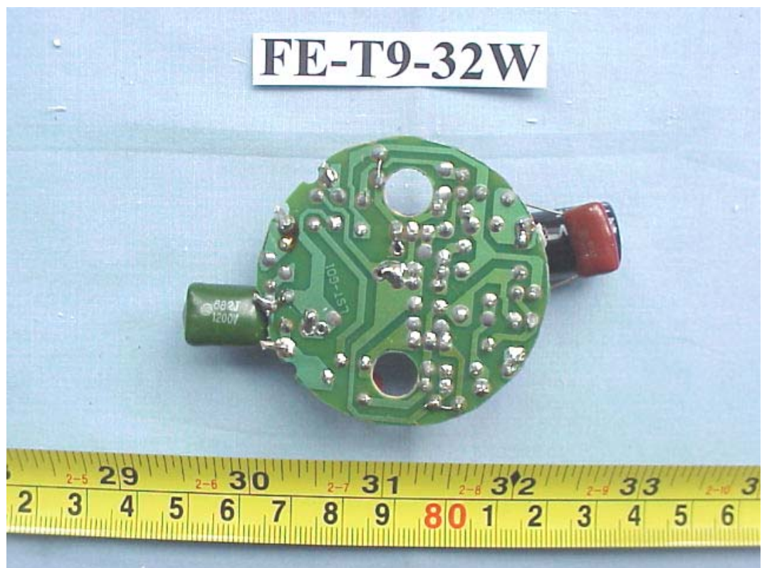
FIGURE 47 ENERGY SAVING LAMP (M/N: FE-T9-32W) MAIN BOARD (SOLDERED SIDE)
