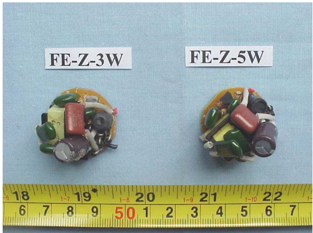
FIGURE 3 ENERGY SAVING LAMP (M/N: FE-Z-3/5W) MAIN BOARD (COMPONENT SIDE)
