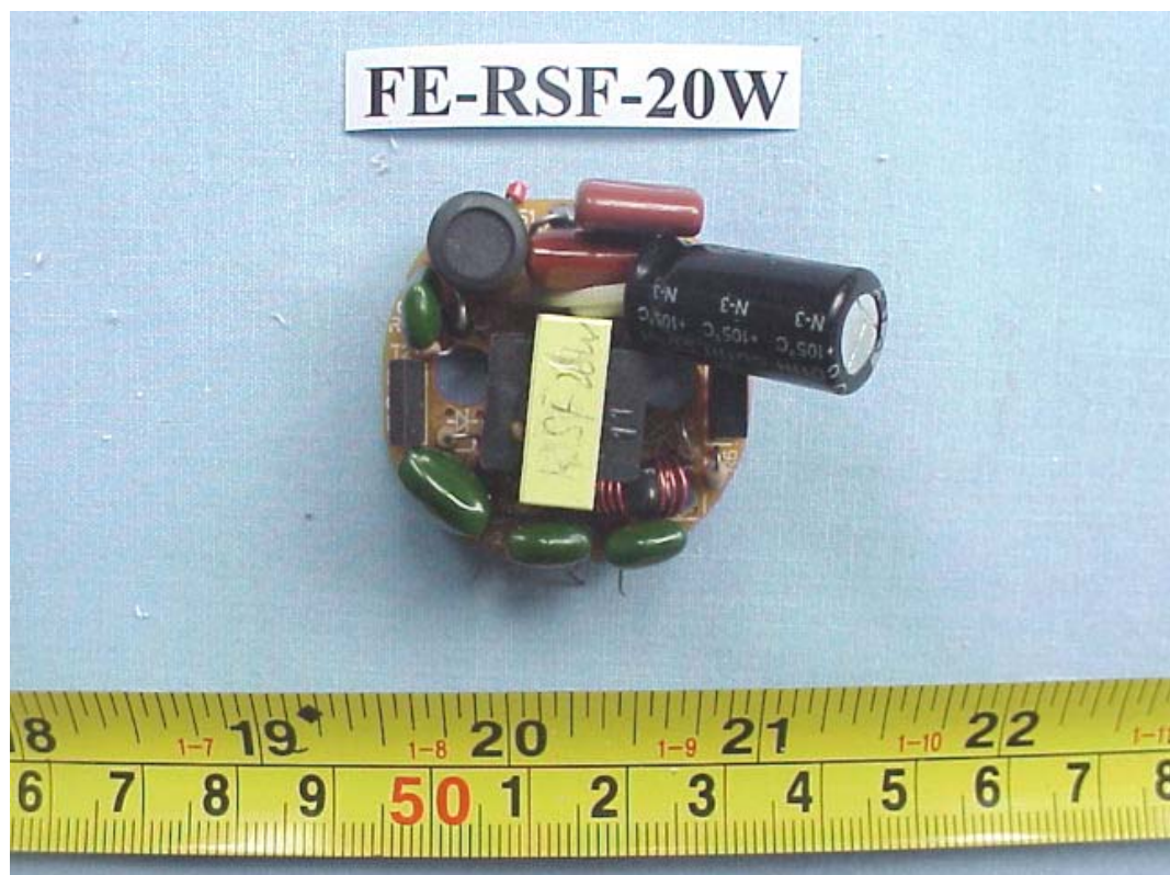
FIGURE 18 ENERGY SAVING LAMP (M/N: FE-RSF-20W) MAIN BOARD (COMPONENT SIDE)
