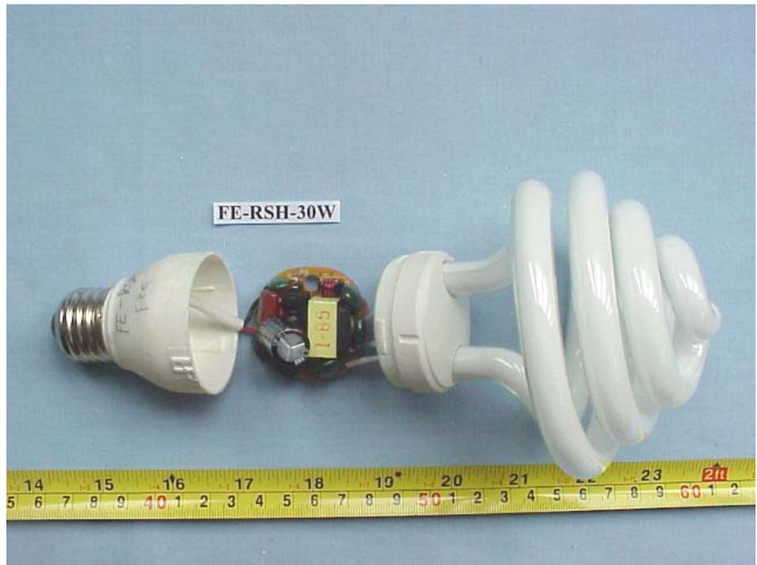
FIGURE 33 ENERGY SAVING LAMP (M/N: FE-RSH-30W) COVER REMOVED 2
