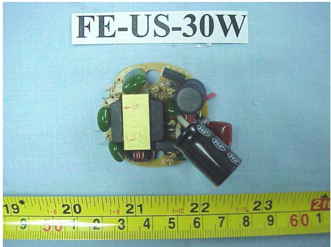
FIGURE 43 ENERGY SAVING LAMP (M/N: FE-US-30W) MAIN BOARD (COMPONENT SIDE)
