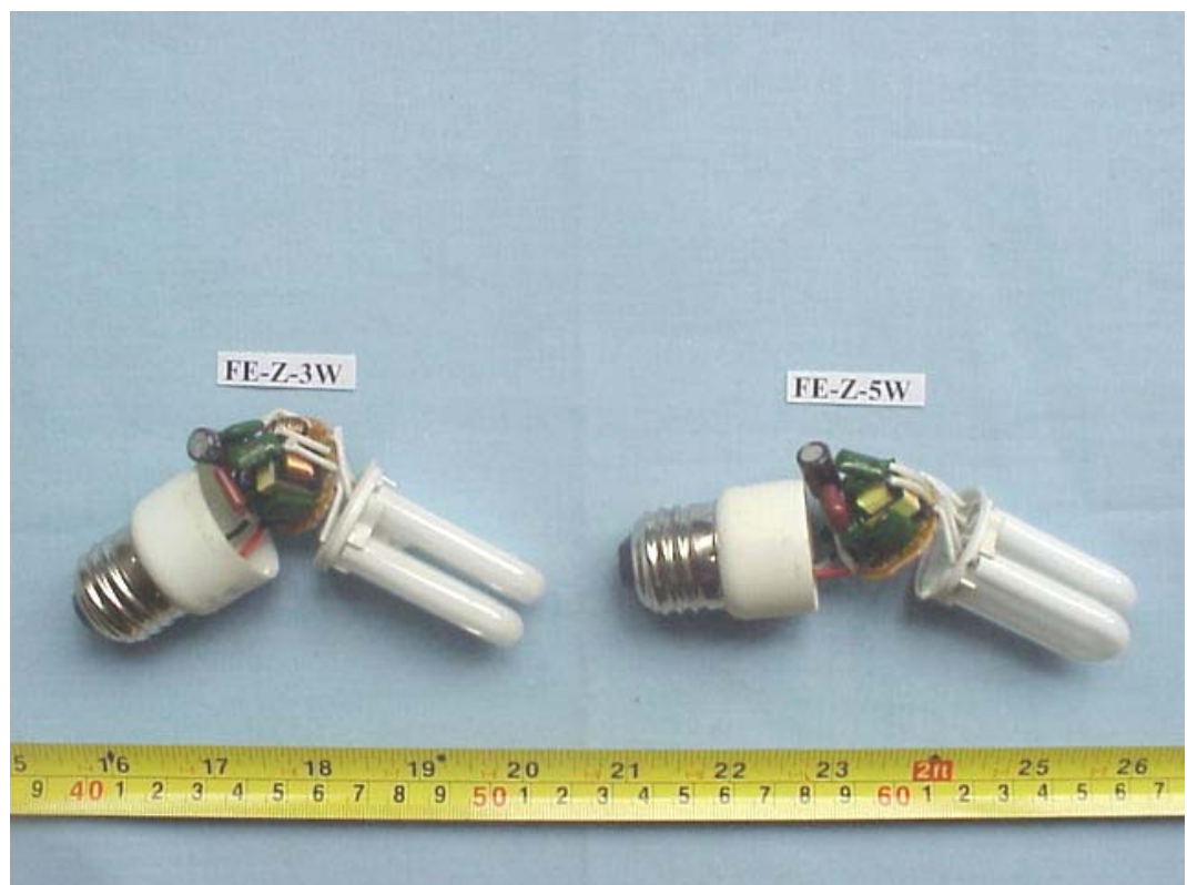
FIGURE 2 ENERGY SAVING LAMP (M/N: FE-Z-3/5W) COVER REMOVED 2
