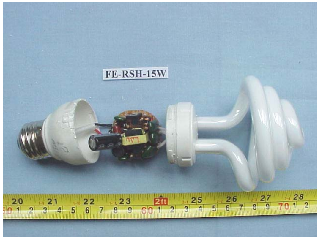
FIGURE 25 ENERGY SAVING LAMP (M/N: FE-RSH-15W) COVER REMOVED 2
