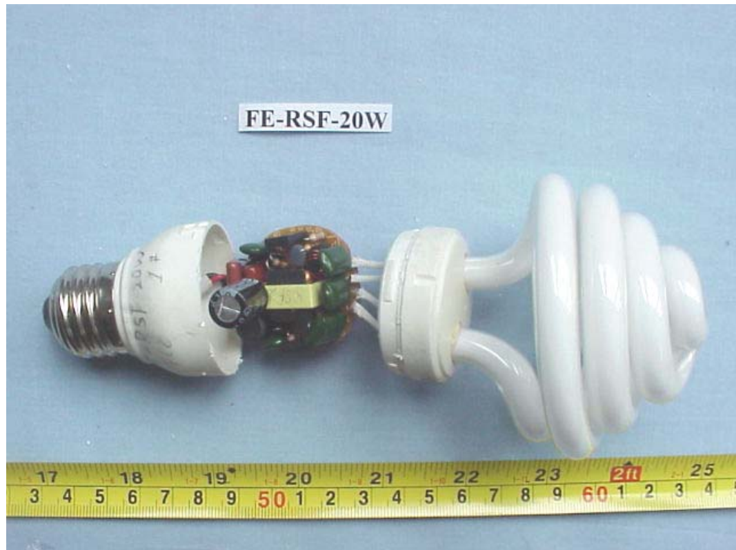
FIGURE 17 ENERGY SAVING LAMP (M/N: FE-RSF-20W) COVER REMOVED 2
