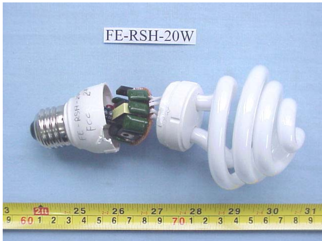
FIGURE 29 ENERGY SAVING LAMP (M/N: FE-RSH-20W) COVER REMOVED 2
