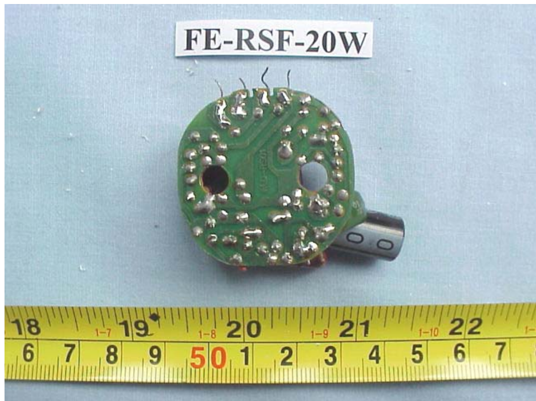
FIGURE 19 ENERGY SAVING LAMP (M/N: FE-RSF-20W) MAIN BOARD (SOLDERED SIDE)
