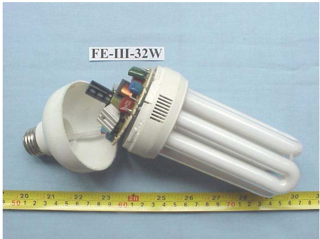
FIGURE 45 ENERGY SAVING LAMP (M/N: FE-III-32W) COVER REMOVED
