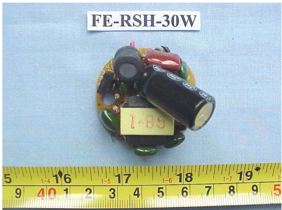
FIGURE 34 ENERGY SAVING LAMP (M/N: FE-RSH-30W) MAIN BOARD (COMPONENT SIDE)
