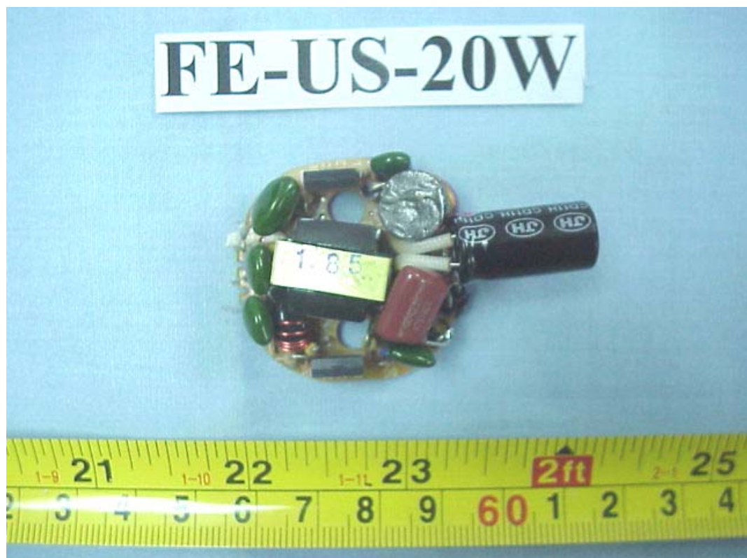
FIGURE 40 ENERGY SAVING LAMP (M/N: FE-US-20W) MAIN BOARD (COMPONENT SIDE)
