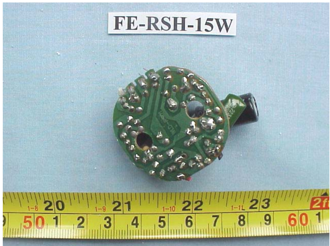
FIGURE 27 ENERGY SAVING LAMP (M/N: FE-RSH-15W) MAIN BOARD (SOLDERED SIDE)
