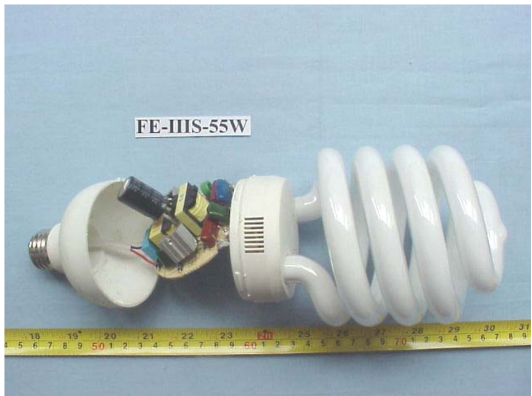
FIGURE 60 ENERGY SAVING LAMP (M/N: FE-IIIIS-55W) COVER REMOVED
