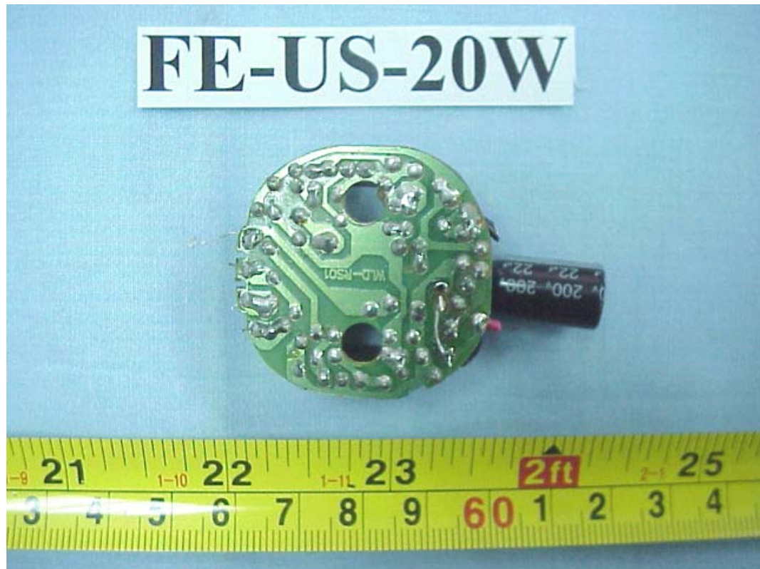
FIGURE 41 ENERGY SAVING LAMP (M/N: FE-US-20W) MAIN BOARD (SOLDERED SIDE)
