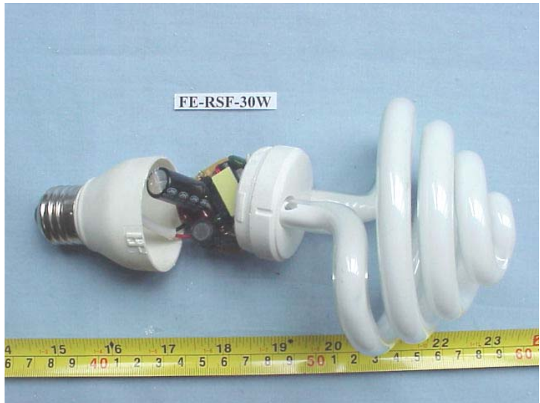
FIGURE 21 ENERGY SAVING LAMP (M/N: FE-RSF-30W) COVER REMOVED 2
