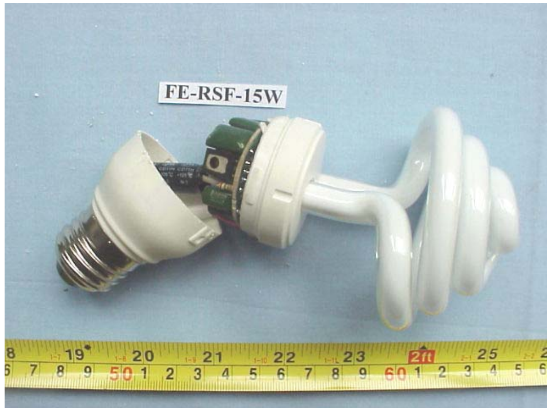
FIGURE 13 ENERGY SAVING LAMP (M/N: FE-RSF-15W) COVER REMOVED
