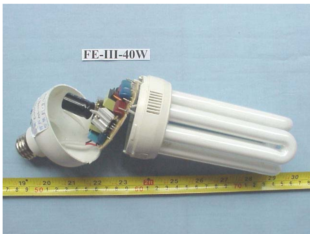
FIGURE 48 ENERGY SAVING LAMP (M/N: FE-III-40W) COVER REMOVED
