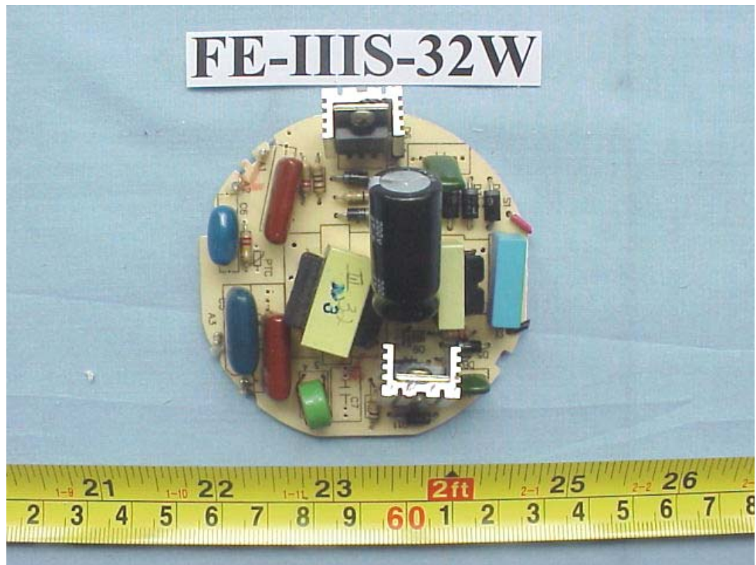
FIGURE 55 ENERGY SAVING LAMP (M/N: FE-IIIIS-32W) MAIN BOARD (COMPONENT SIDE)
