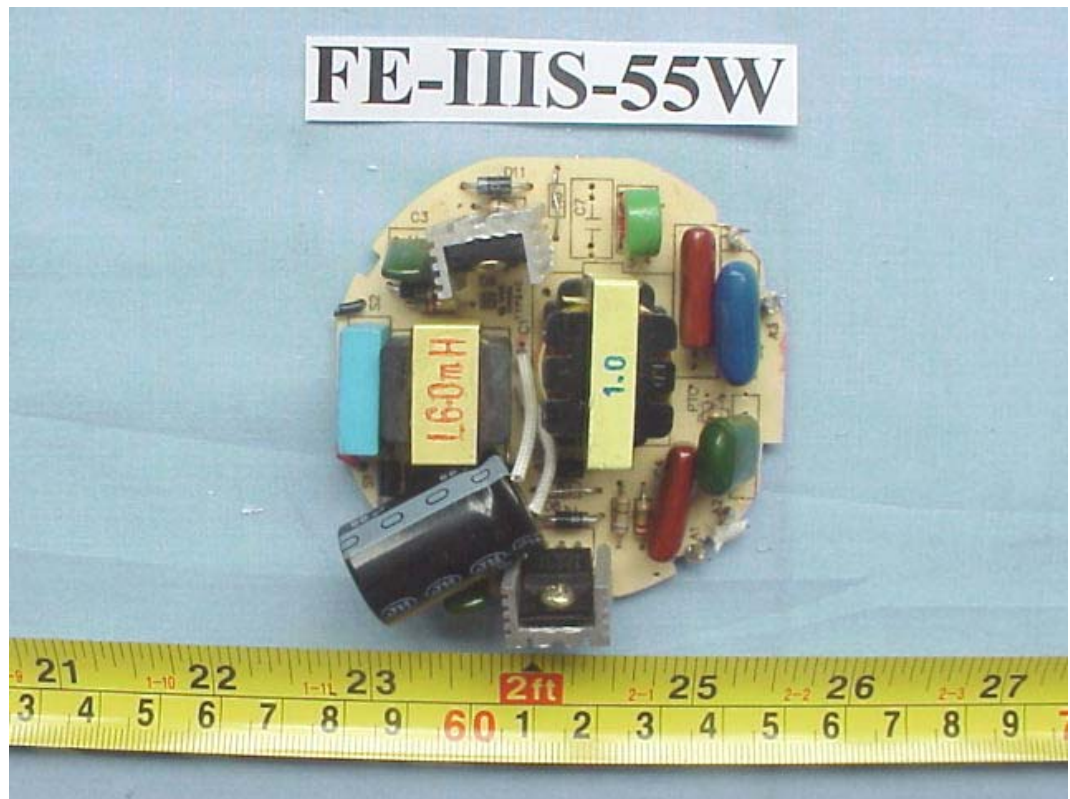
FIGURE 61 ENERGY SAVING LAMP (M/N: FE-IIIIS-55W) MAIN BOARD (COMPONENT SIDE)
