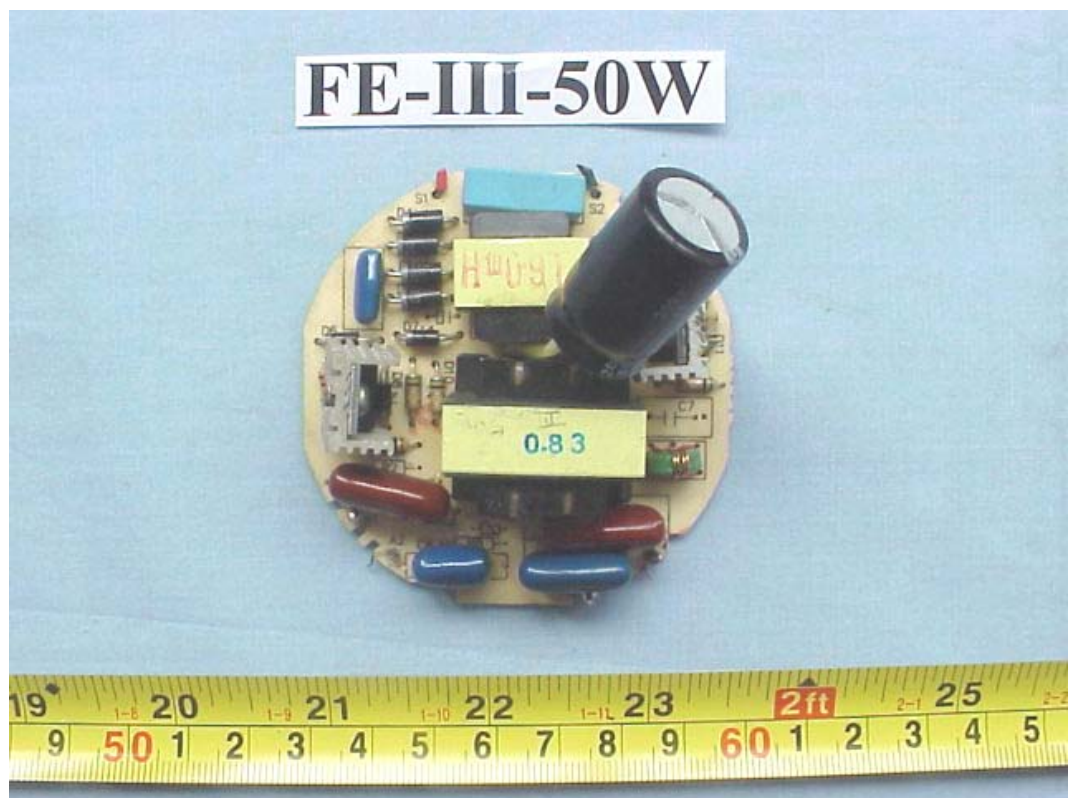
FIGURE 52 ENERGY SAVING LAMP (M/N: FE-III-50W) MAIN BOARD (COMPONENT SIDE)
