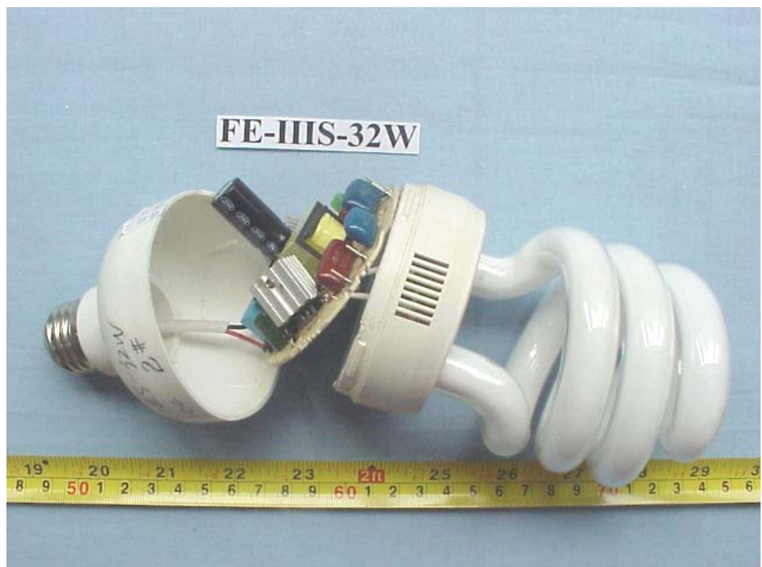
FIGURE 54 ENERGY SAVING LAMP (M/N: FE-IIIIS-32W) COVER REMOVED
