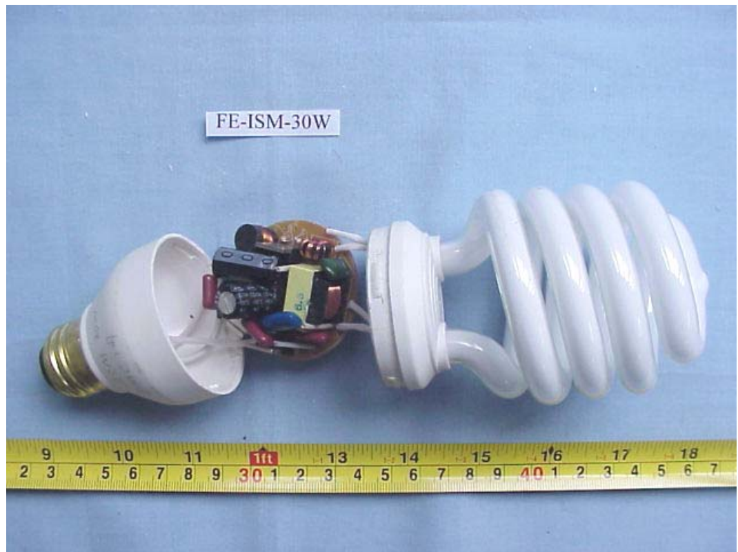
FIGURE 40 ENERGY SAVING LAMP (M/N: FE-ISM-30W) COVER REMOVED
