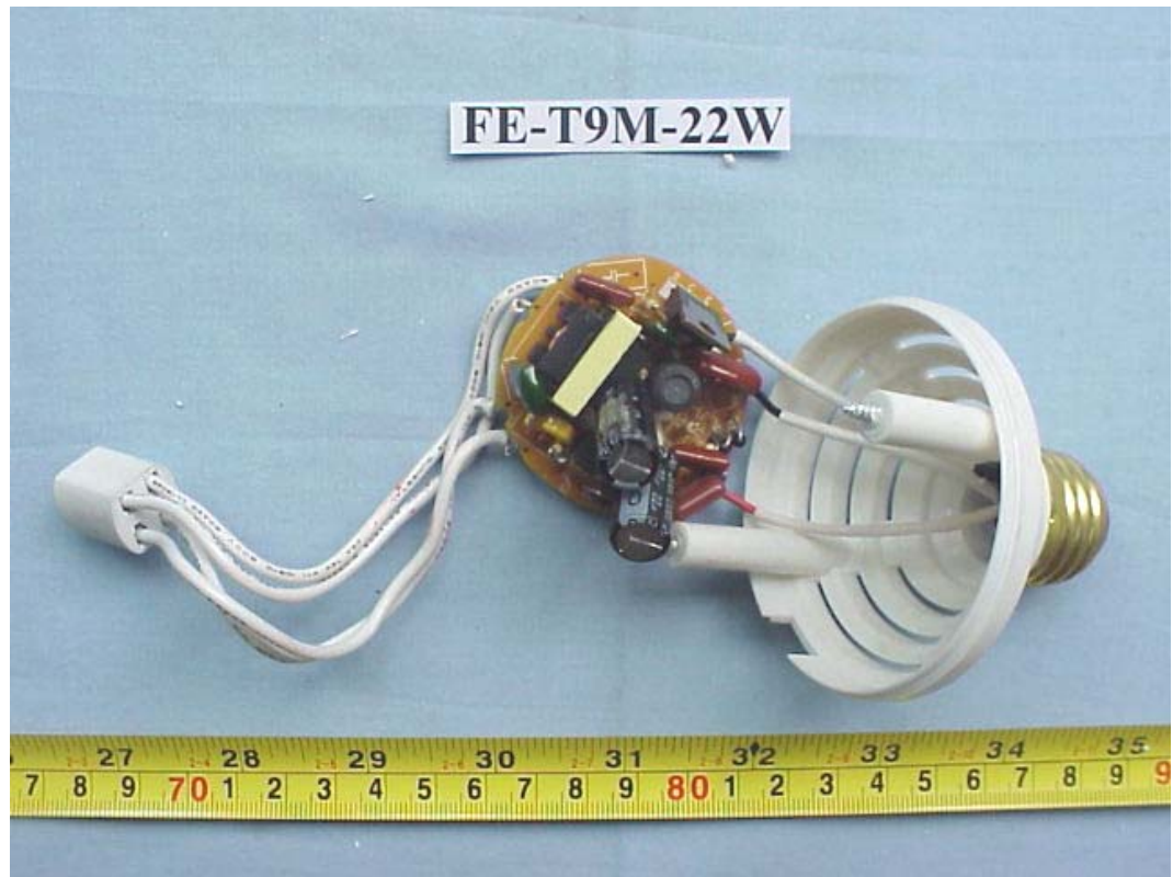
FIGURE 43 ENERGY SAVING LAMP (M/N: FE-T9M-22W) COVER REMOVED
