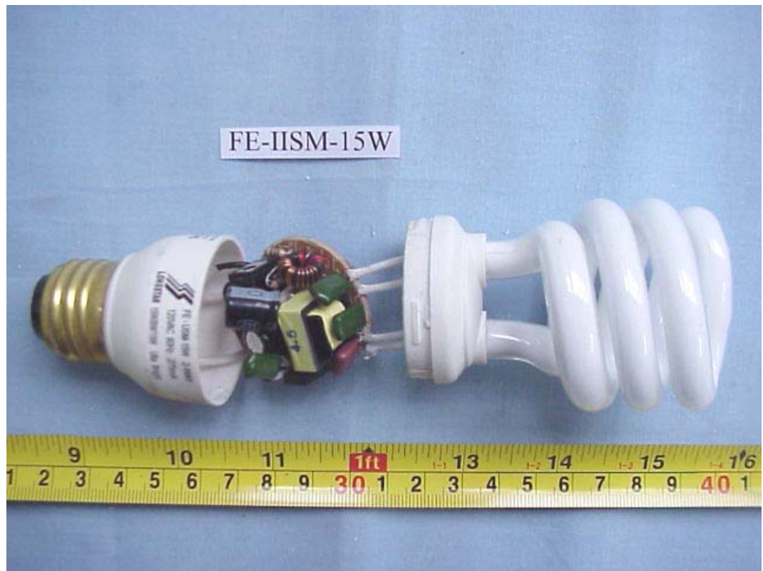
FIGURE 4 ENERGY SAVING LAMP (M/N: FE-IIISM-15W) COVER REMOVED
