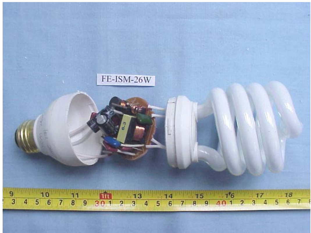
FIGURE 37 ENERGY SAVING LAMP (M/N: FE-ISM-26W) COVER REMOVED
