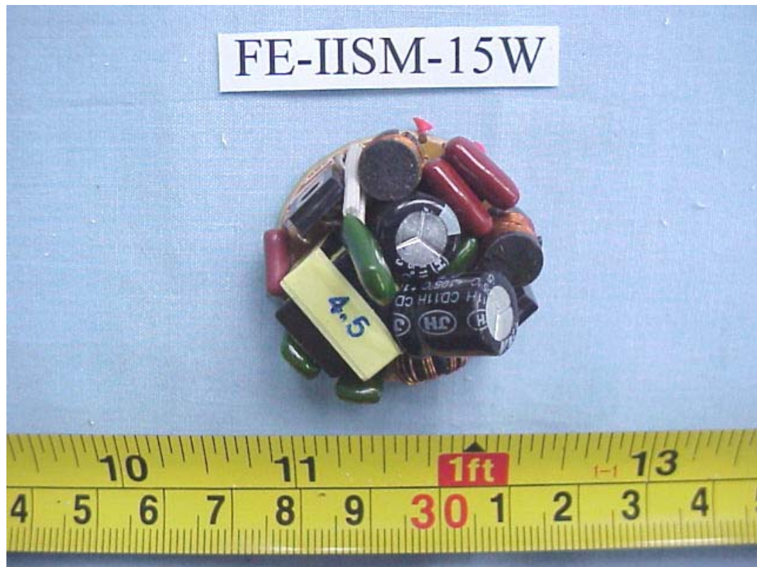
FIGURE 5 ENERGY SAVING LAMP (M/N: FE-IISM-15W) MAIN BOARD (COMPONENT SIDE)
