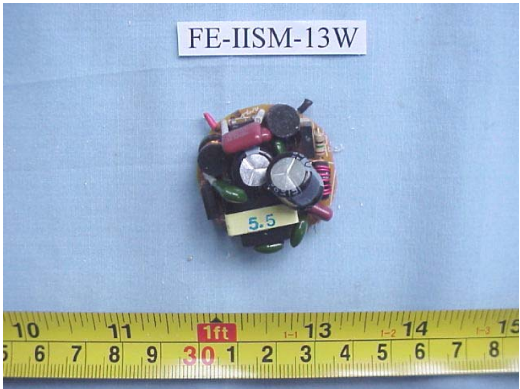
FIGURE 2 ENERGY SAVING LAMP (M/N: FE-IISM-13W) MAIN BOARD (COMPONENT SIDE)
