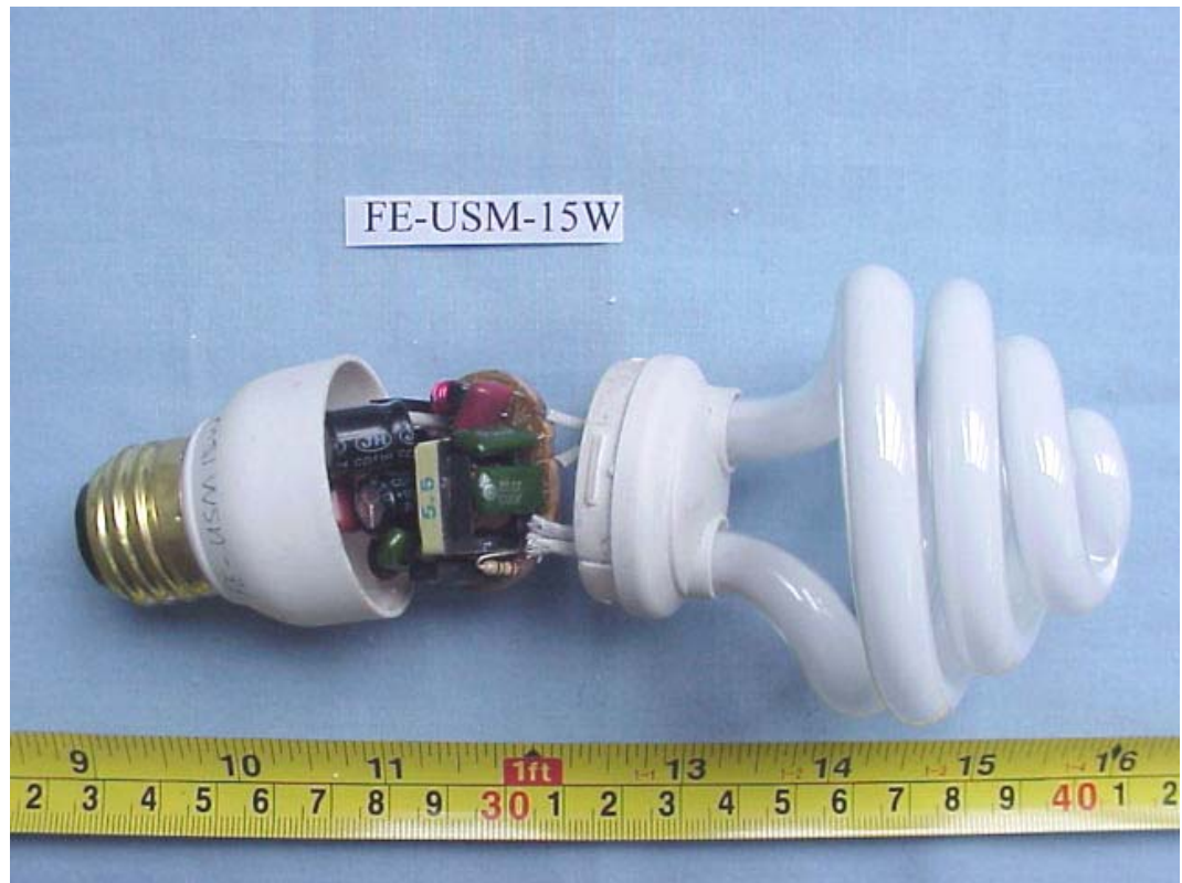
FIGURE 13 ENERGY SAVING LAMP (M/N: FE-USM-15W) COVER REMOVED
