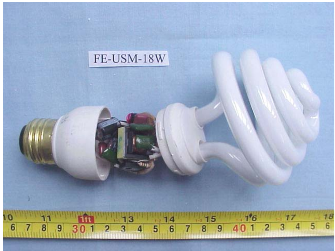
FIGURE 16 ENERGY SAVING LAMP (M/N: FE-USM-18W) COVER REMOVED
