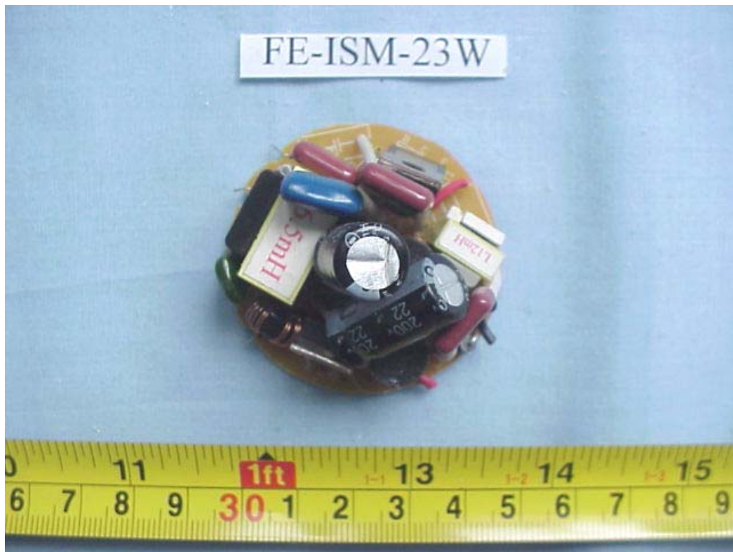
FIGURE 35 ENERGY SAVING LAMP (M/N: FE-ISM-23W) MAIN BOARD (COMPONENT SIDE)
