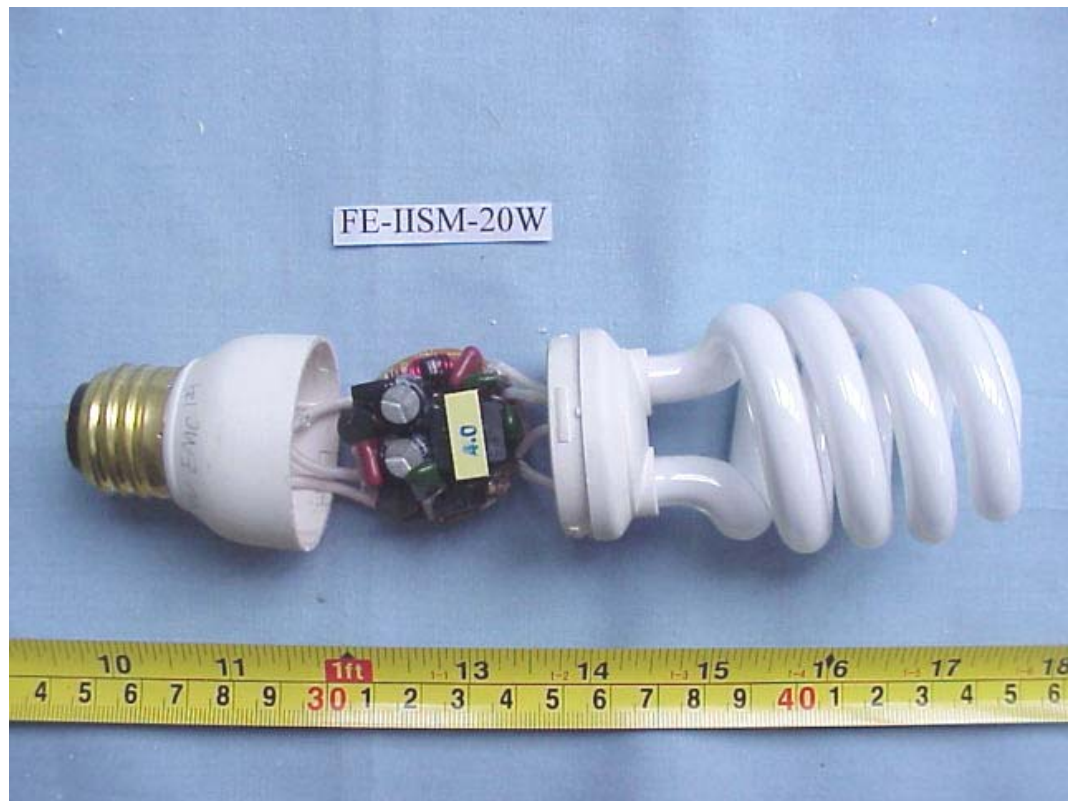
FIGURE 10 ENERGY SAVING LAMP (M/N: FE-IISM-20W) COVER REMOVED
