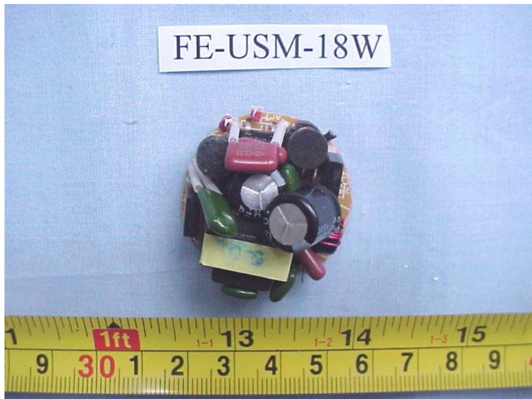
FIGURE 17 ENERGY SAVING LAMP (M/N: FE-USM-18W) MAIN BOARD (COMPONENT SIDE)
