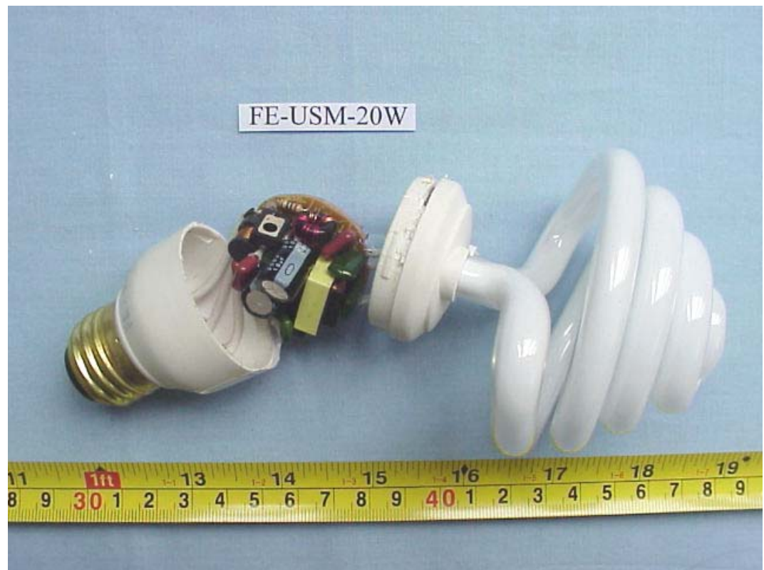
FIGURE 19 ENERGY SAVING LAMP (M/N: FE-USM-20W) COVER REMOVED
