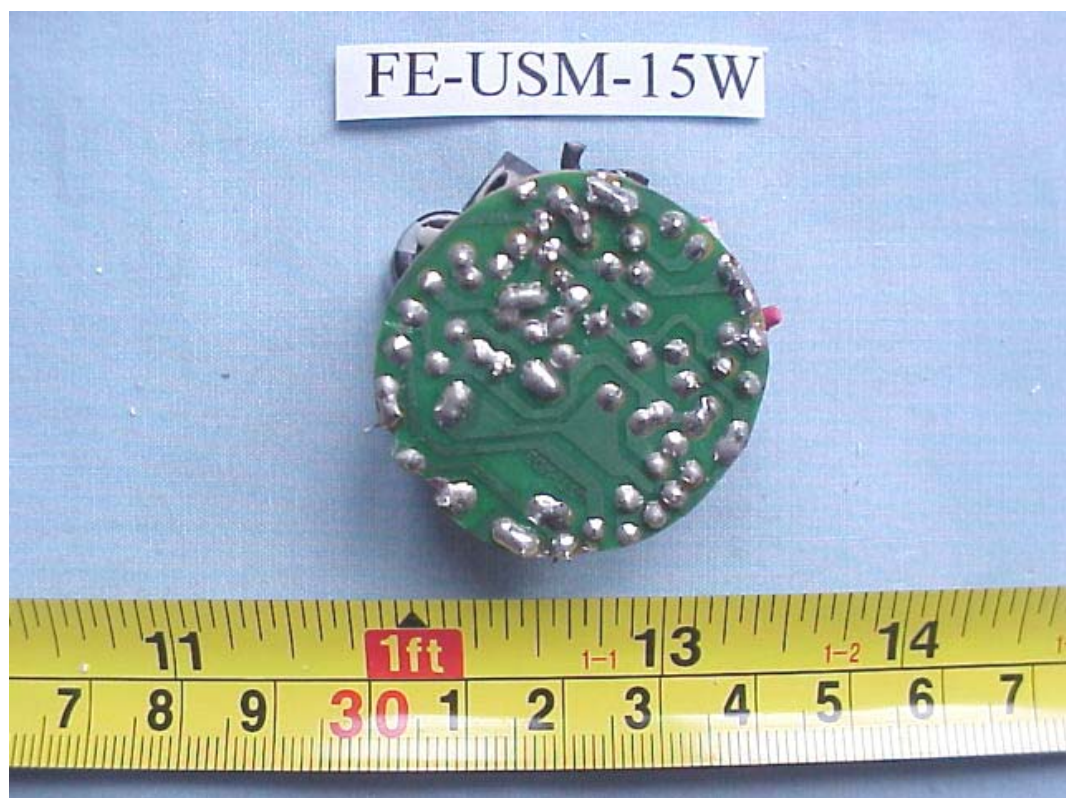
FIGURE 15 ENERGY SAVING LAMP (M/N: FE-USM-15W) MAIN BOARD (SOLDERED SIDE)
