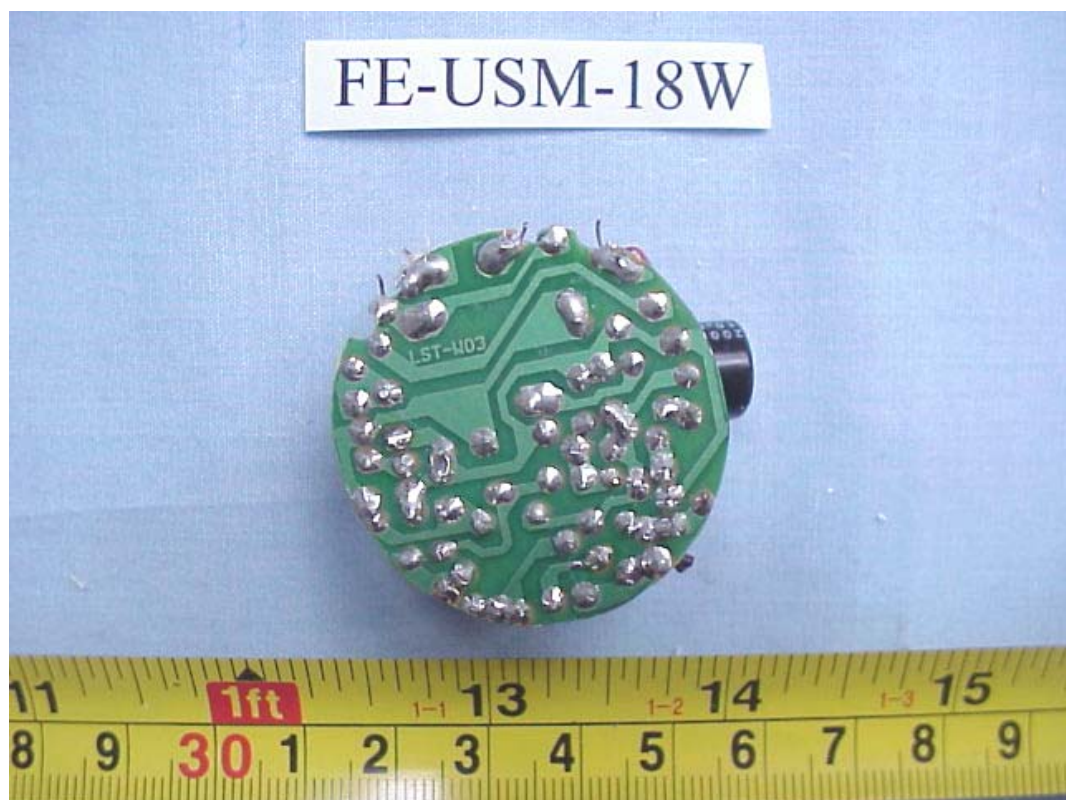
FIGURE 18 ENERGY SAVING LAMP (M/N: FE-USM-18W) MAIN BOARD (SOLDERED SIDE)
