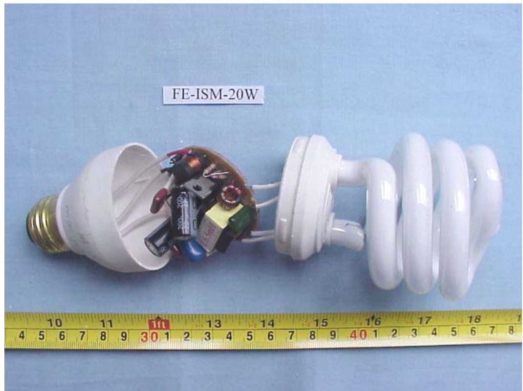
FIGURE 31 ENERGY SAVING LAMP (M/N: FE-ISM-20W) COVER REMOVED
