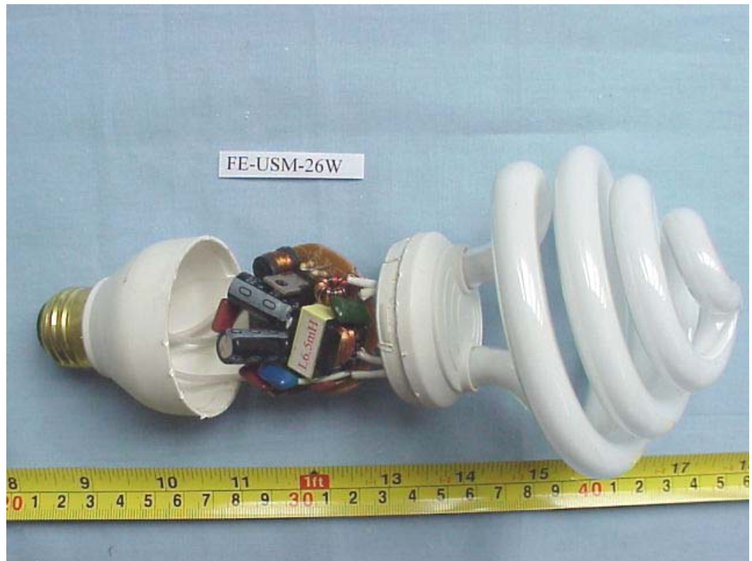
FIGURE 25 ENERGY SAVING LAMP (M/N: FE-USM-26W) COVER REMOVED
