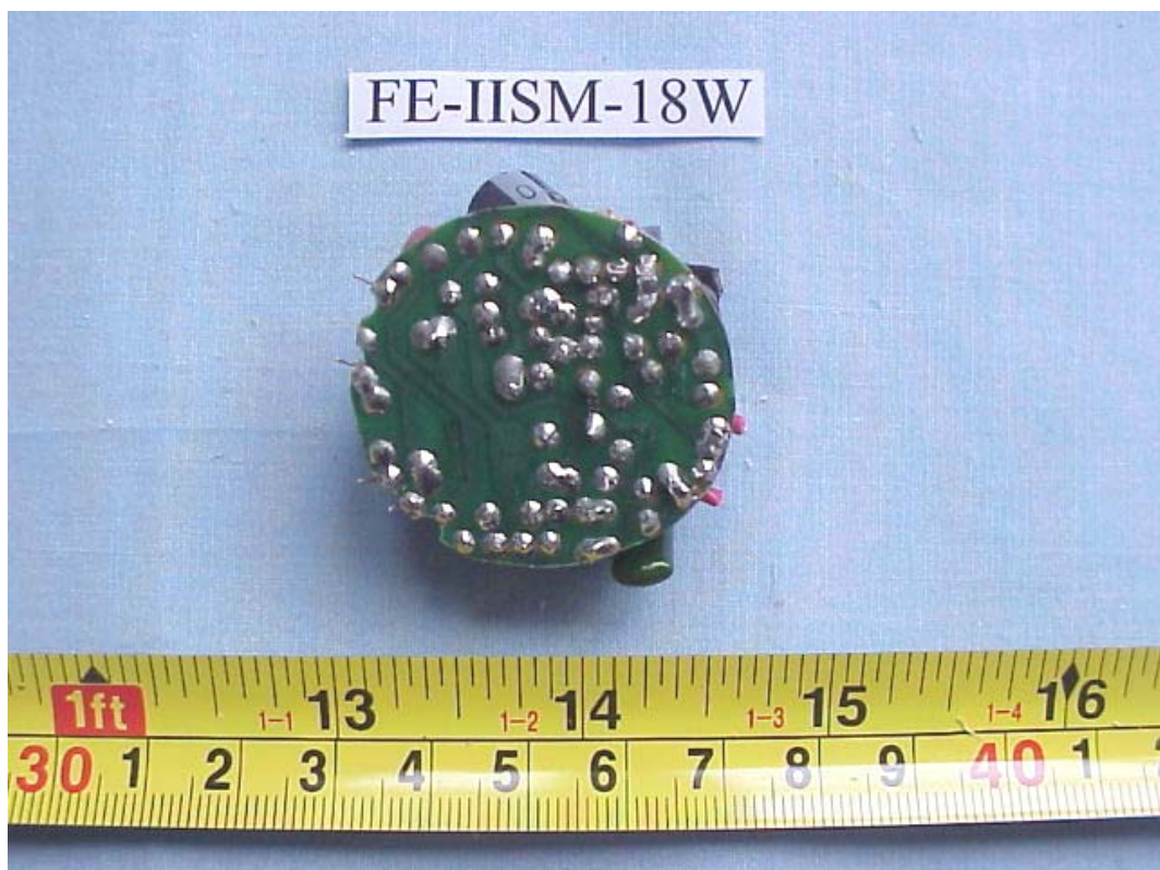
FIGURE 9 ENERGY SAVING LAMP (M/N: FE-IISM-18W) MAIN BOARD (SOLDERED SIDE)
