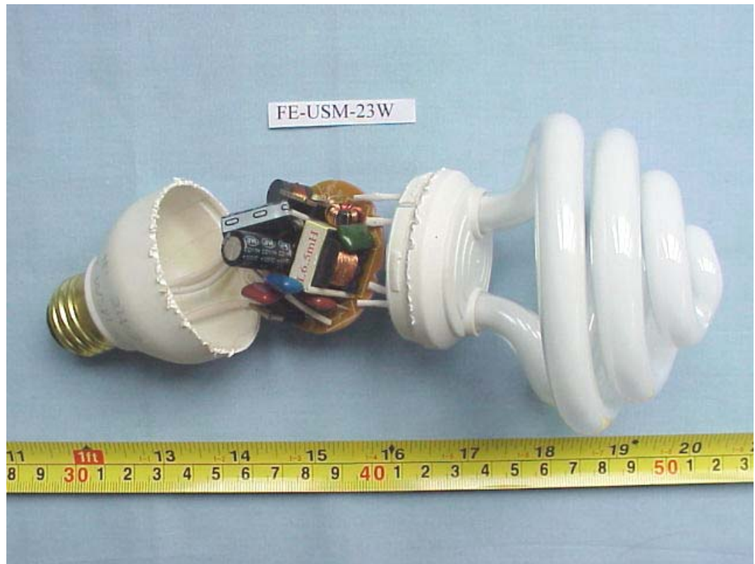
FIGURE 22 ENERGY SAVING LAMP (M/N: FE-USM-23W) COVER REMOVED
