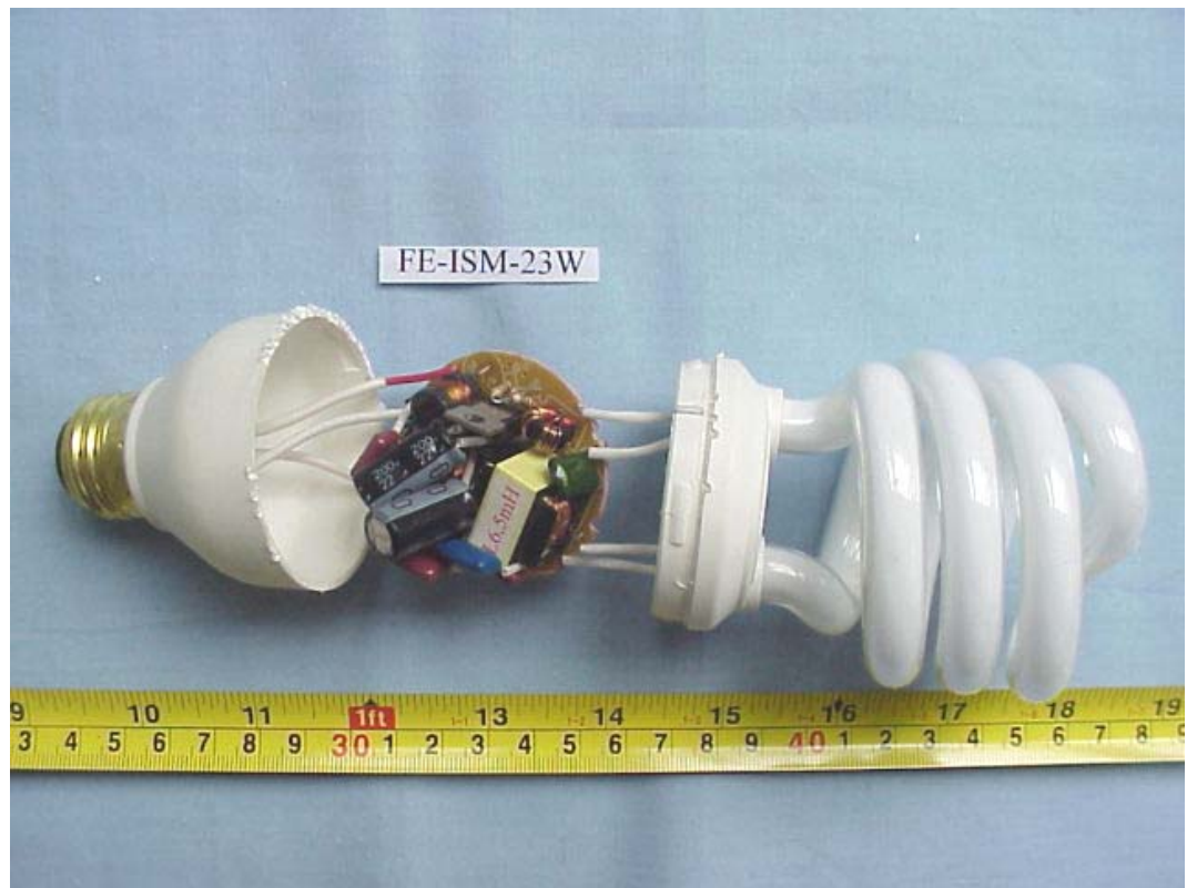
FIGURE 34 ENERGY SAVING LAMP (M/N: FE-ISM-23W) COVER REMOVED
