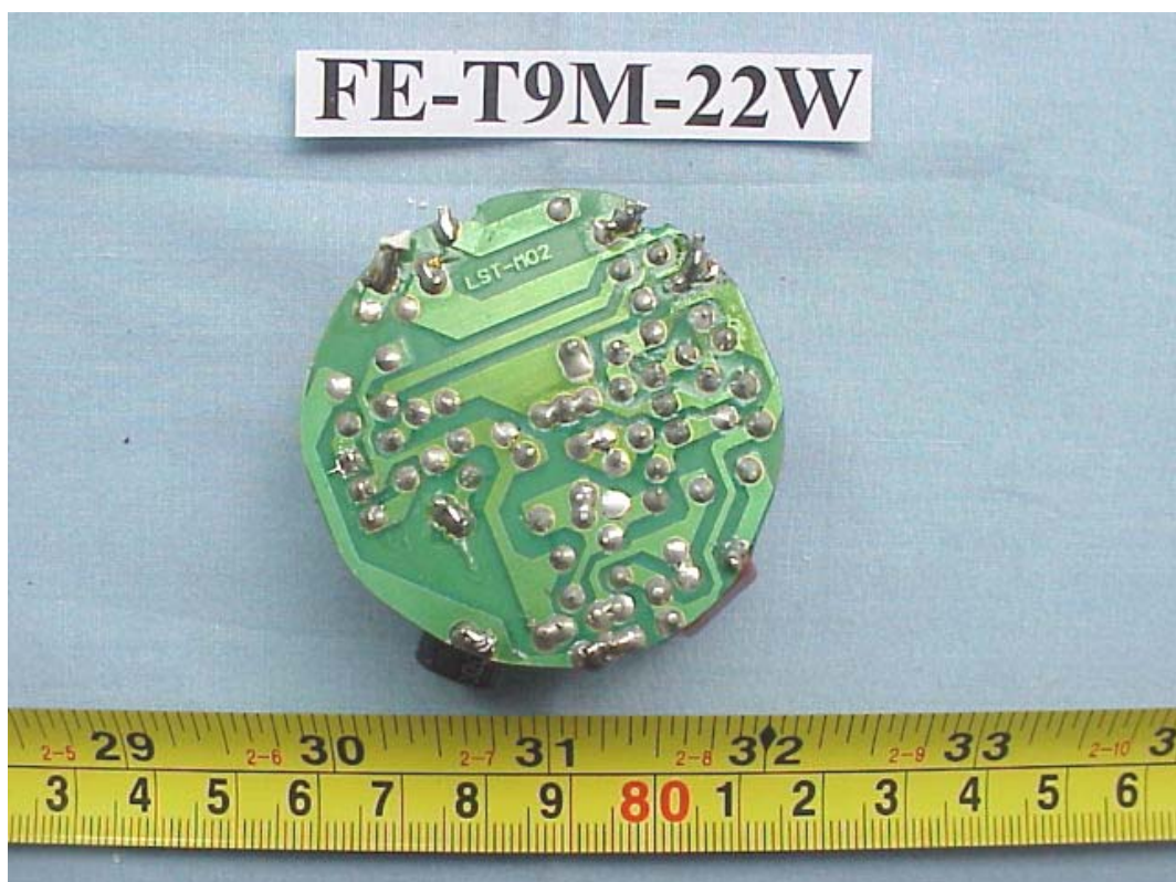
FIGURE 45 ENERGY SAVING LAMP (M/N: FE-T9M-22W) MAIN BOARD (SOLDERED SIDE)
