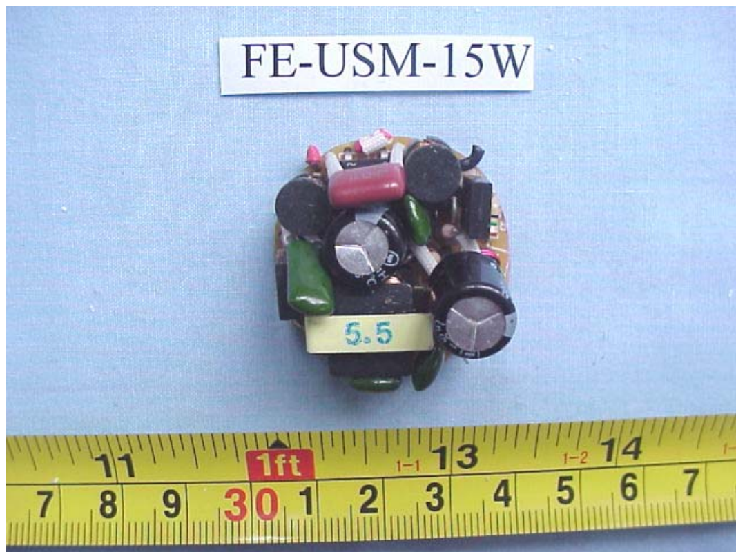
FIGURE 14 ENERGY SAVING LAMP (M/N: FE-USM-15W) MAIN BOARD (COMPONENT SIDE)
