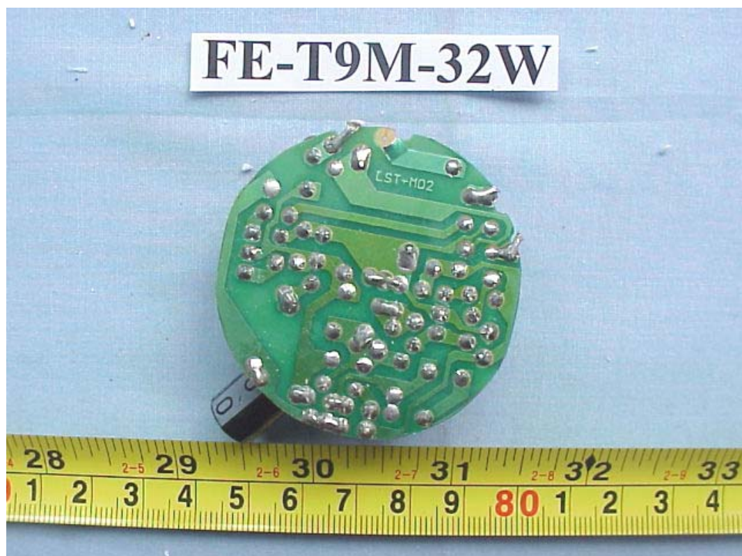
FIGURE 48 ENERGY SAVING LAMP (M/N: FE-T9M-32W) MAIN BOARD (SOLDERED SIDE)
