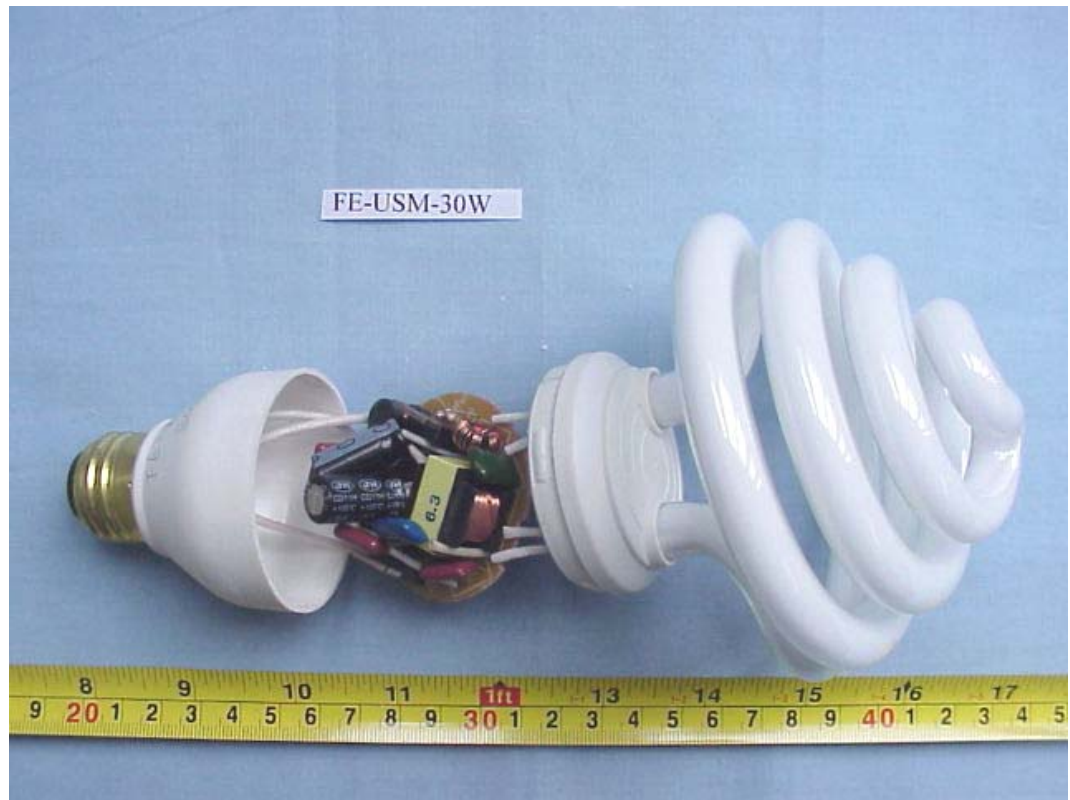
FIGURE 28 ENERGY SAVING LAMP (M/N: FE-USM-30W) COVER REMOVED
