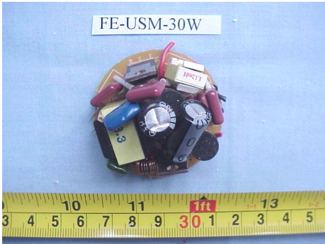
FIGURE 29 ENERGY SAVING LAMP (M/N: FE-USM-30W) MAIN BOARD (COMPONENT SIDE)
