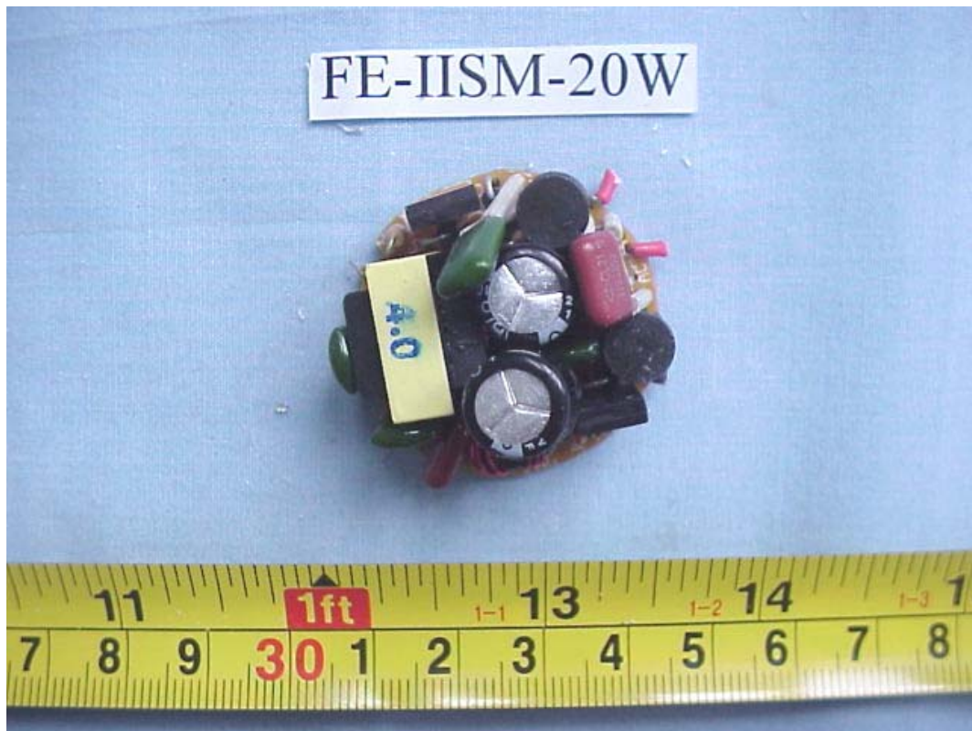
FIGURE 11 ENERGY SAVING LAMP (M/N: FE-IISM-20W) MAIN BOARD (COMPONENT SIDE)
