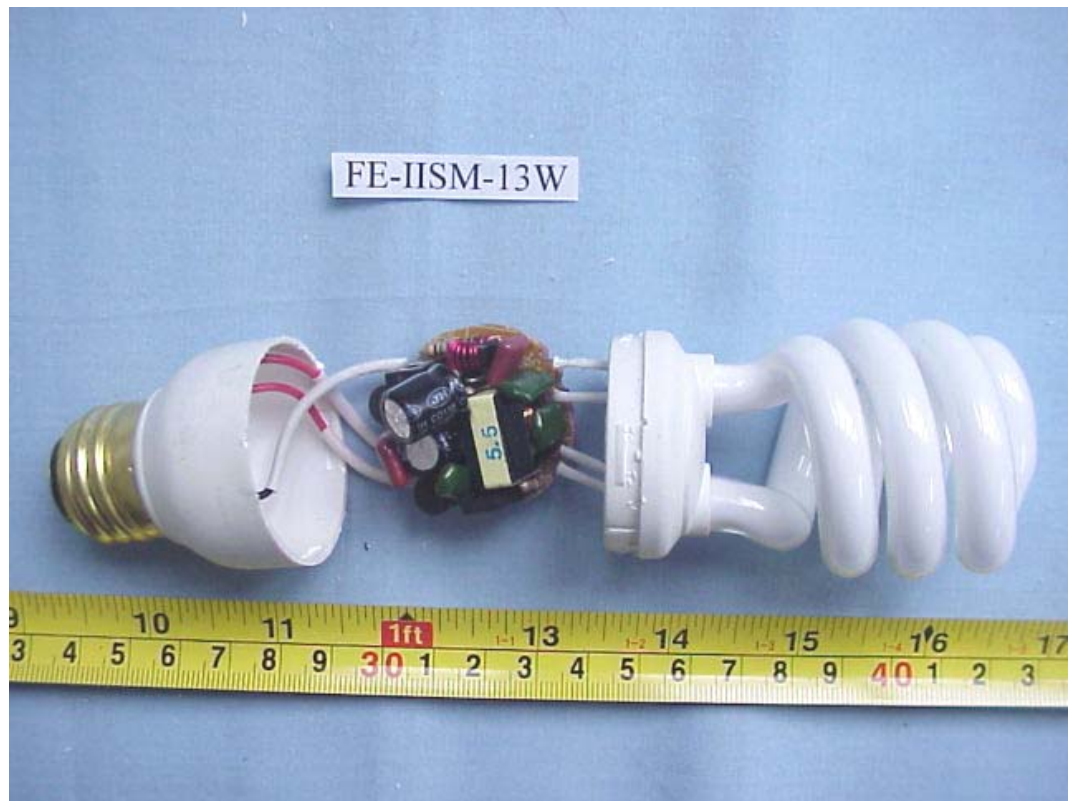
FIGURE 1 ENERGY SAVING LAMP (M/N: FE-IIISM-13W) COVER REMOVED
