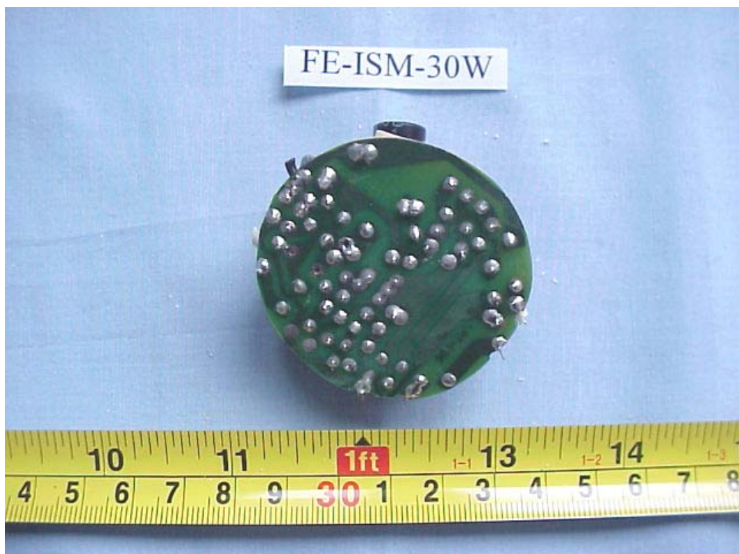
FIGURE 42 ENERGY SAVING LAMP (M/N: FE-ISM-30W) MAIN BOARD (SOLDERED SIDE)
