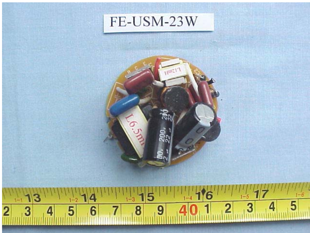
FIGURE 23 ENERGY SAVING LAMP (M/N: FE-USM-23W) MAIN BOARD (COMPONENT SIDE)
