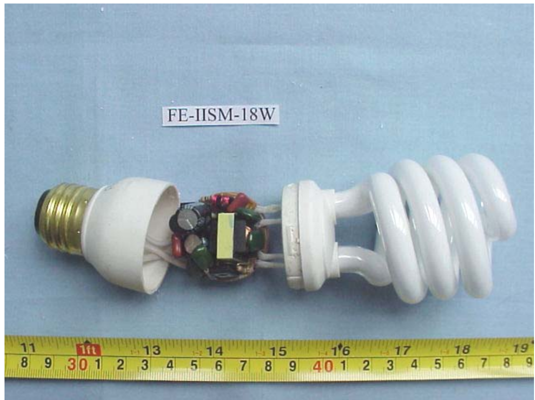
FIGURE 7 ENERGY SAVING LAMP (M/N: FE-IISM-18W) COVER REMOVED
