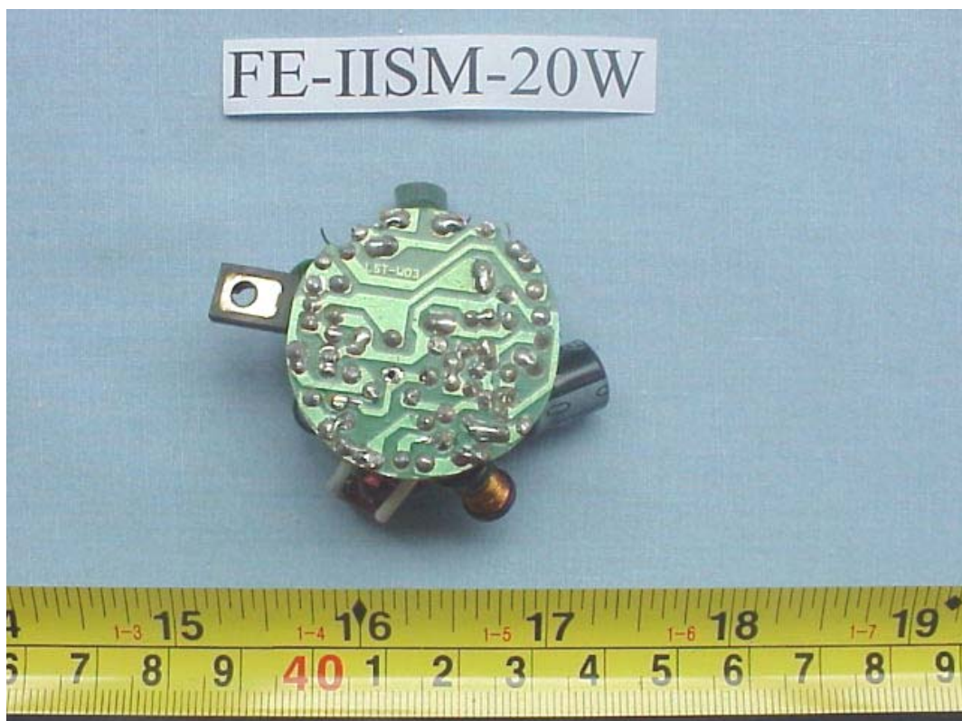
FIGURE 12 ENERGY SAVING LAMP (M/N: FE-IISM-20W) MAIN BOARD (SOLDERED SIDE)
