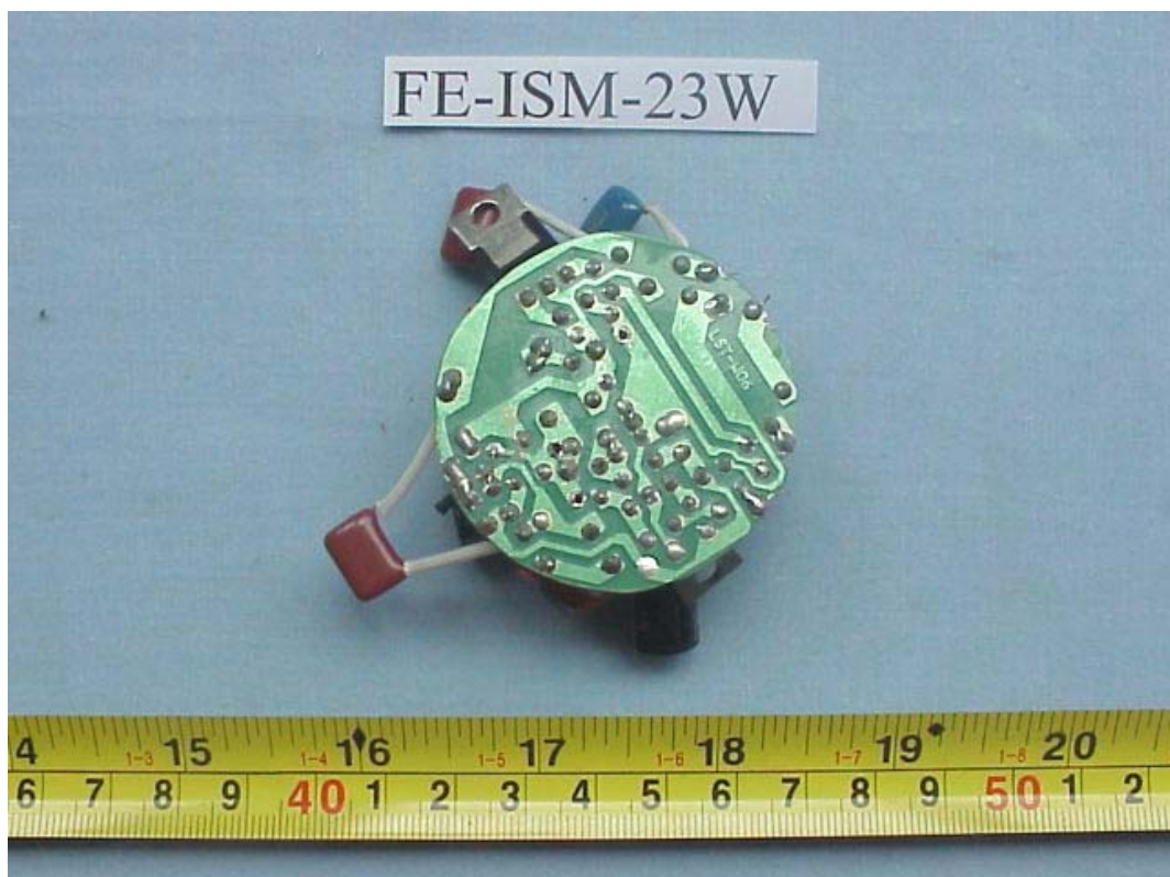
FIGURE 36 ENERGY SAVING LAMP (M/N: FE-ISM-23W) MAIN BOARD (SOLDERED SIDE)
