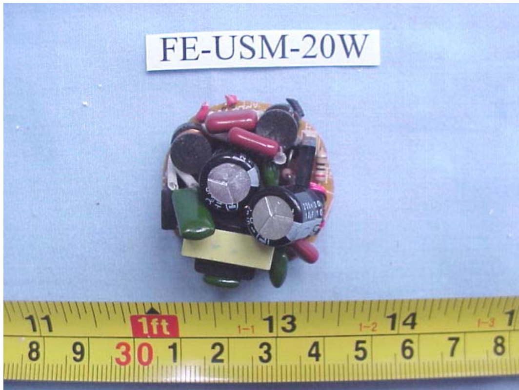
FIGURE 20 ENERGY SAVING LAMP (M/N: FE-USM-20W) MAIN BOARD (COMPONENT SIDE)
