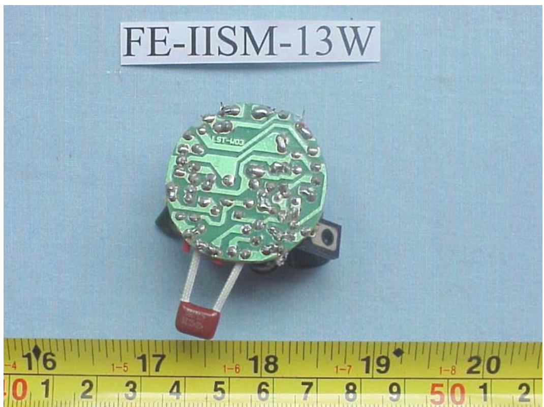
FIGURE 3 ENERGY SAVING LAMP (M/N: FE-IISM-13W) MAIN BOARD (SOLDERED SIDE)
