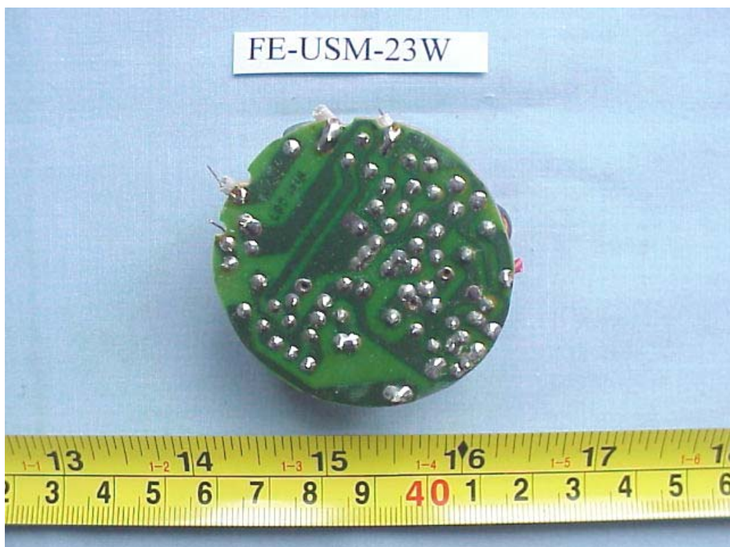
FIGURE 24 ENERGY SAVING LAMP (M/N: FE-USM-23W) MAIN BOARD (SOLDERED SIDE)
