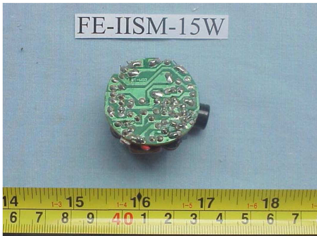
FIGURE 6 ENERGY SAVING LAMP (M/N: FE-IISM-15W) MAIN BOARD (SOLDERED SIDE)
