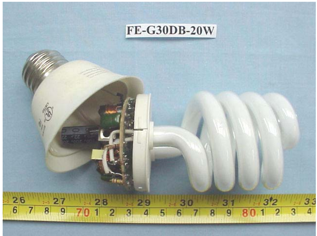
FIGURE 106 ENERGY SAVING LAMP (M/N: FE-G30DB-20W) COVER REMOVED
