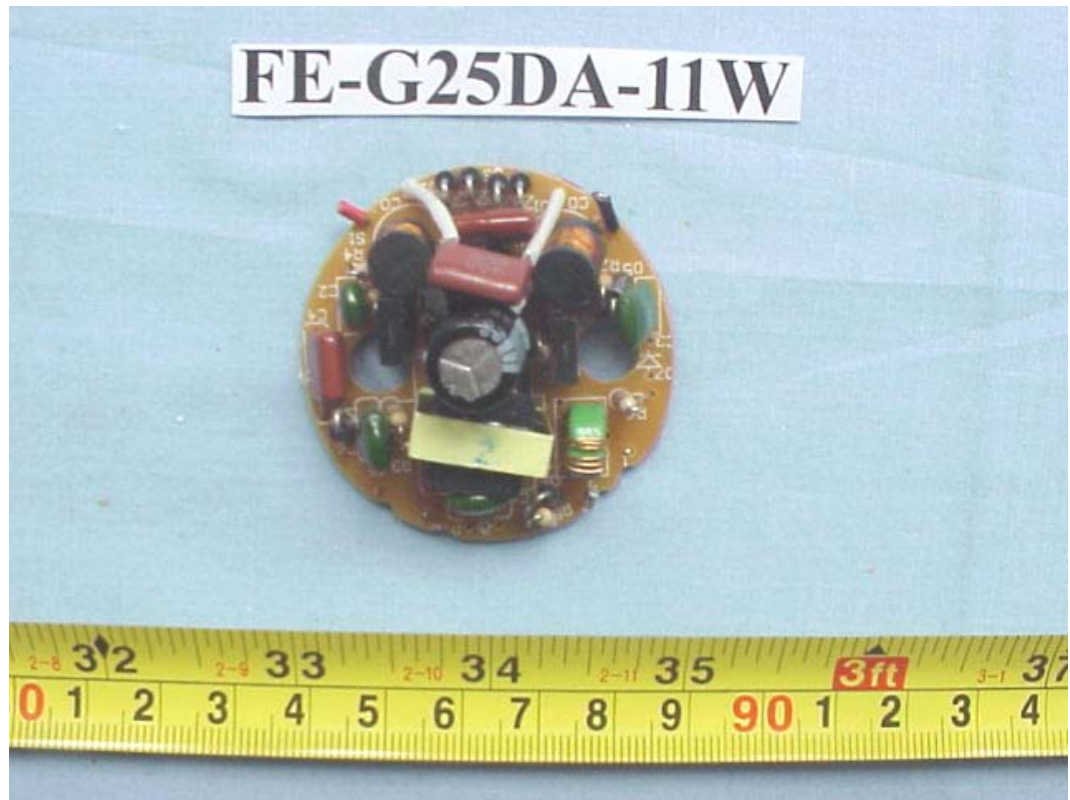
FIGURE 92 ENERGY SAVING LAMP (M/N: FE-G25DA-11W) MAIN BOARD (COMPONENT SIDE)
