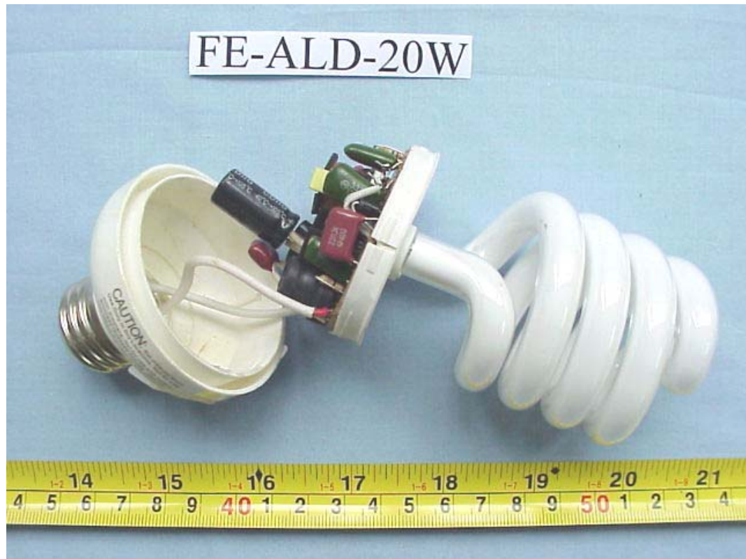
FIGURE 124 ENERGY SAVING LAMP (M/N: FE-ALD-20W) COVER REMOVED
