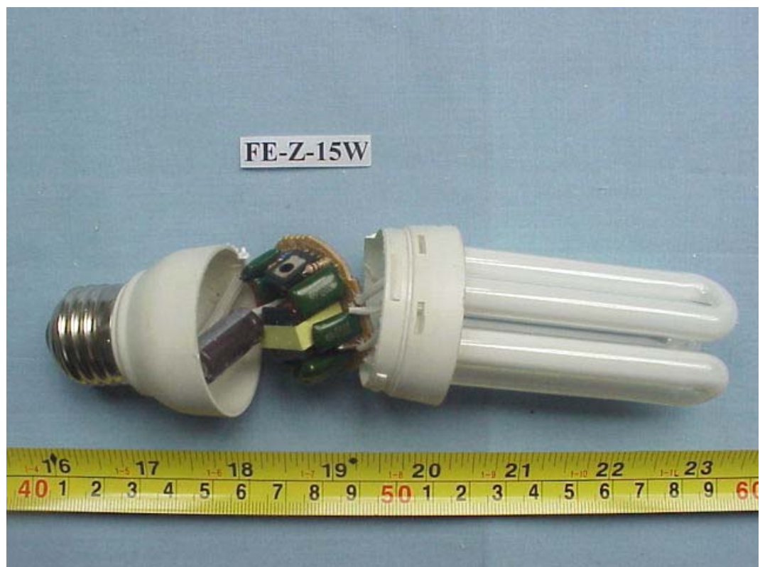
FIGURE 26 ENERGY SAVING LAMP (M/N: FE-Z-15W) COVER REMOVED 2
