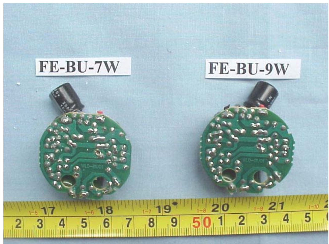
FIGURE 4 ENERGY SAVING LAMP (M/N: FE-BU-7/9W) MAIN BOARD (SOLDERED SIDE)
