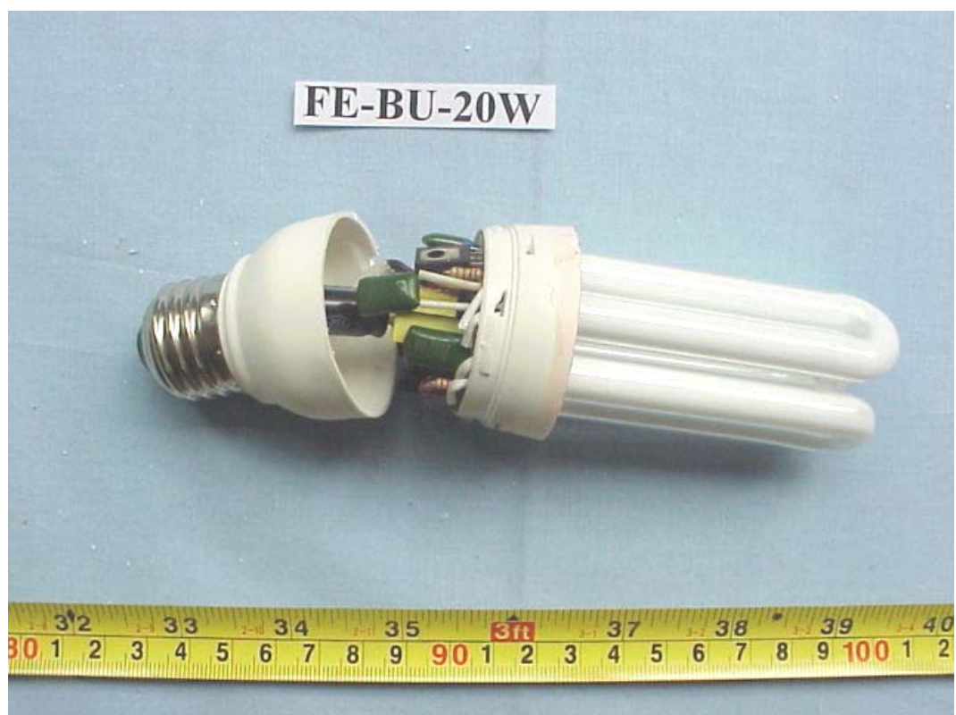
FIGURE 18 ENERGY SAVING LAMP (M/N: FE-BU-20W) COVER REMOVED 2
