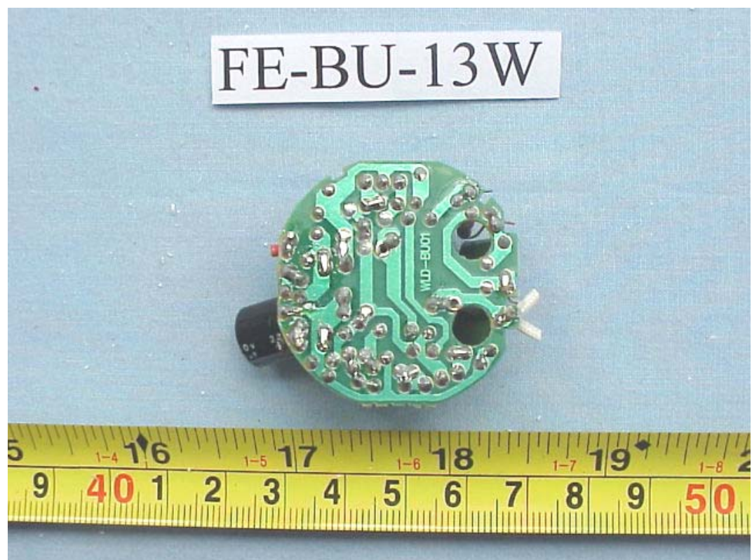
FIGURE 12 ENERGY SAVING LAMP (M/N: FE-BU-13W) MAIN BOARD (SOLDERED SIDE)
