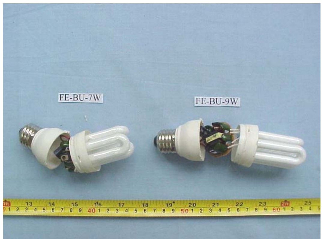
FIGURE 2 ENERGY SAVING LAMP (M/N: FE-BU-7/9W) COVER REMOVED 2
