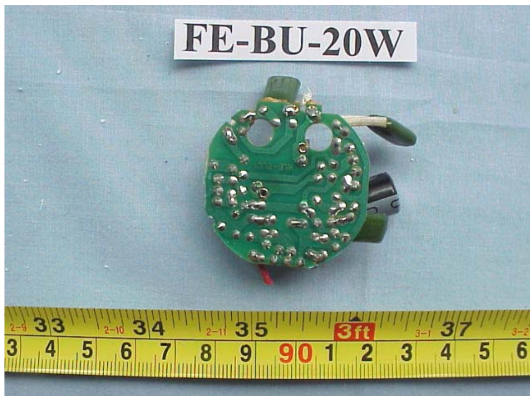
FIGURE 20 ENERGY SAVING LAMP (M/N: FE-BU-20W) MAIN BOARD (SOLDERED SIDE)
