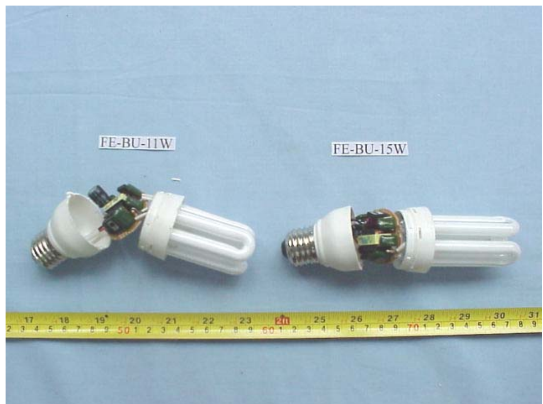
FIGURE 6 ENERGY SAVING LAMP (M/N: FE-BU-11/15W) COVER REMOVED 2
