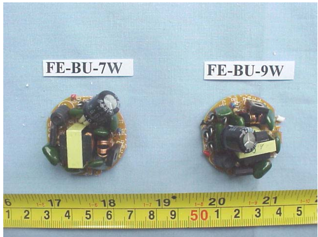
FIGURE 3 ENERGY SAVING LAMP (M/N: FE-BU-7/9W) MAIN BOARD (COMPONENT SIDE)
