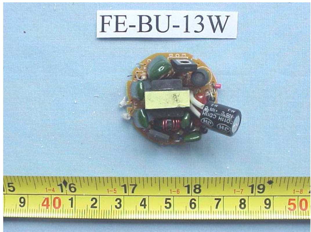
FIGURE 11 ENERGY SAVING LAMP (M/N: FE-BU-13W) MAIN BOARD (COMPONENT SIDE)
