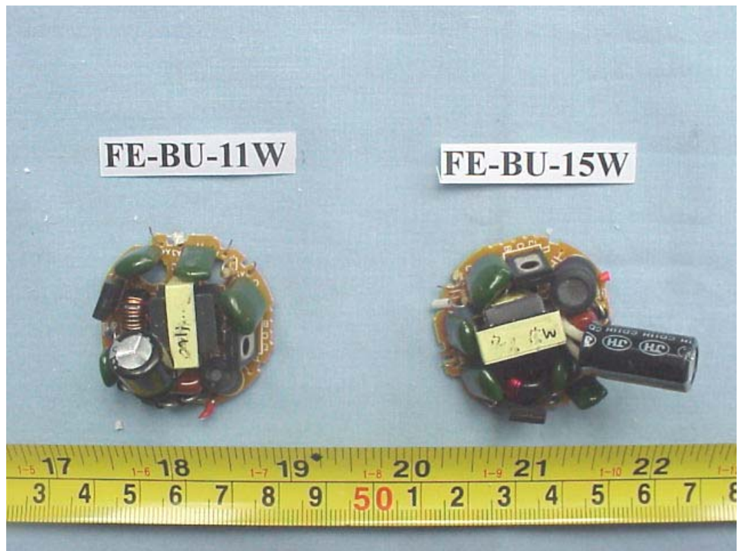
FIGURE 7 ENERGY SAVING LAMP (M/N: FE-BU-11/15W) MAIN BOARD (COMPONENT SIDE)
