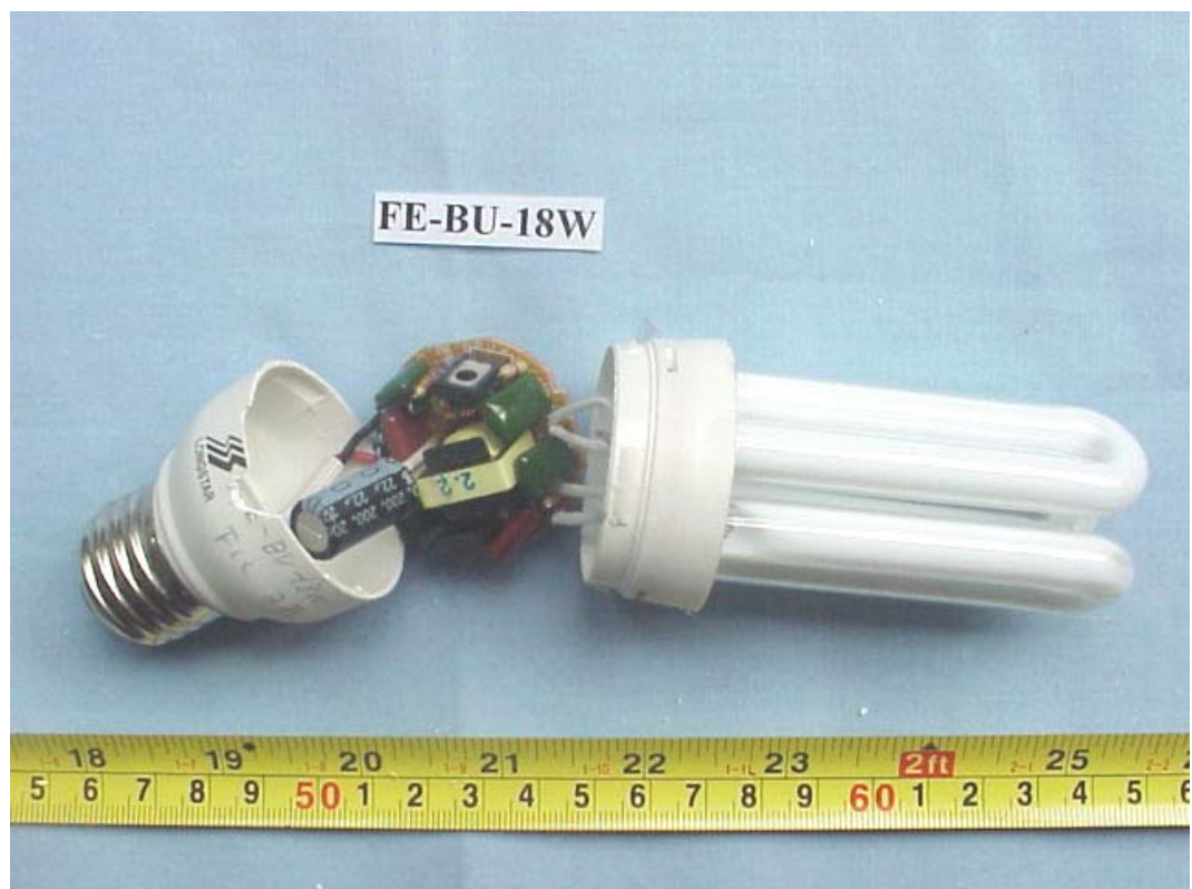
FIGURE 14 ENERGY SAVING LAMP (M/N: FE-BU-18W) COVER REMOVED 2
