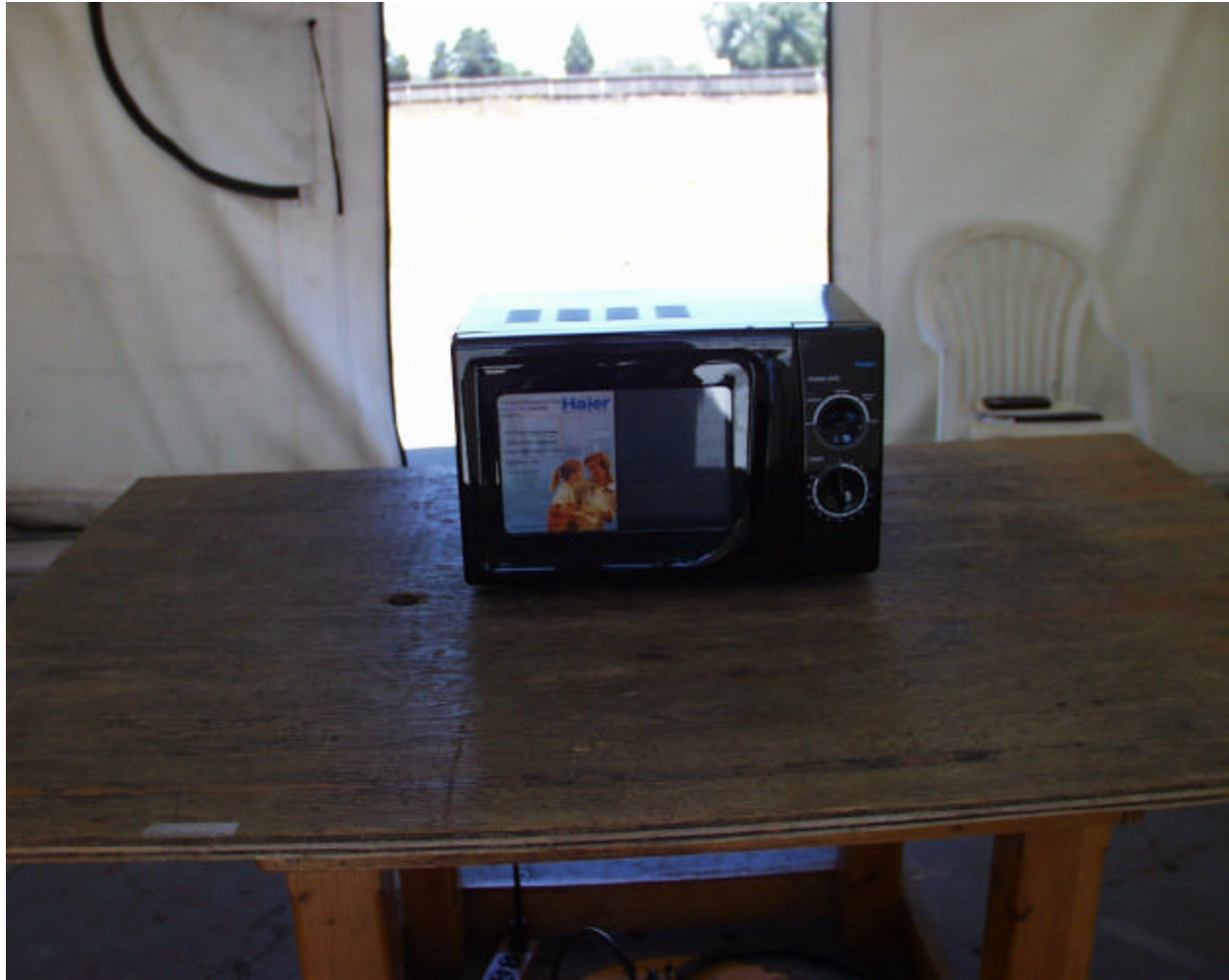
RADIATED TEST SETUP BELOW 1GHz (FRONT SIDE)
