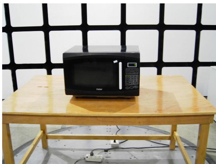
**RADIATED EMISSION TEST SETUP REAR VIEW**
