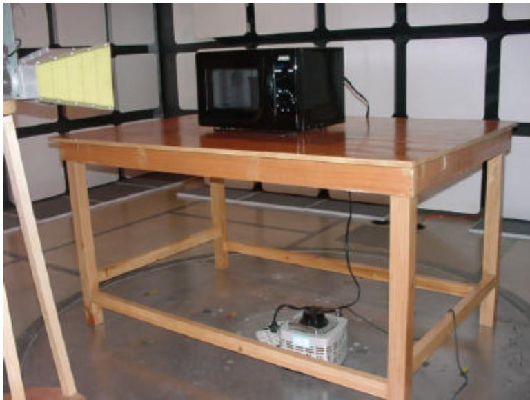
**Leakage Test Setup – Front View**
