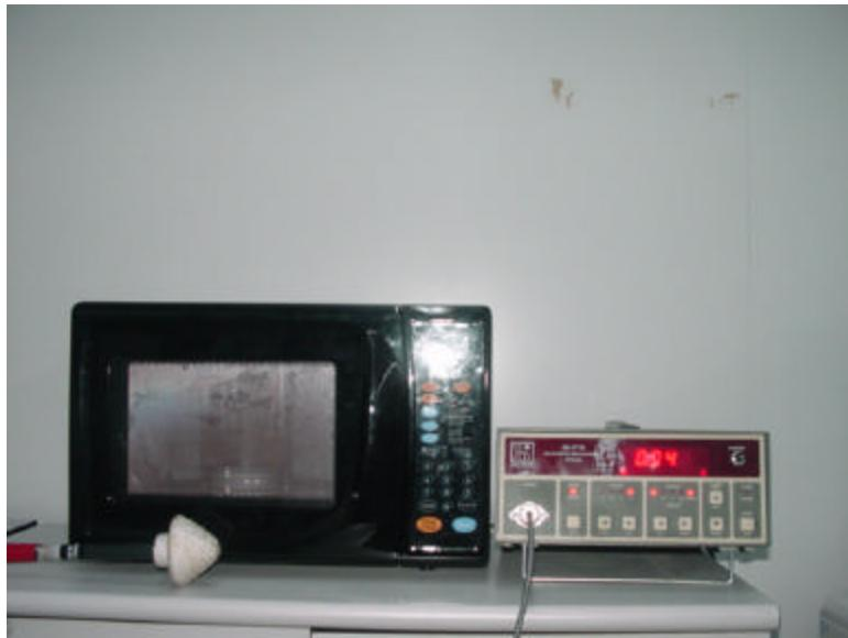
**Input Power Test Setup1 – Front View**
