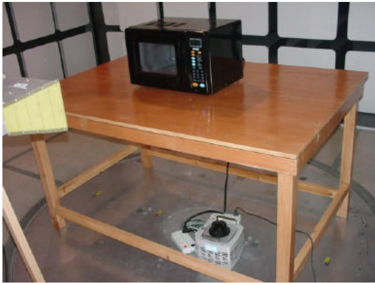
**Leakage Test Setup – Front View**
