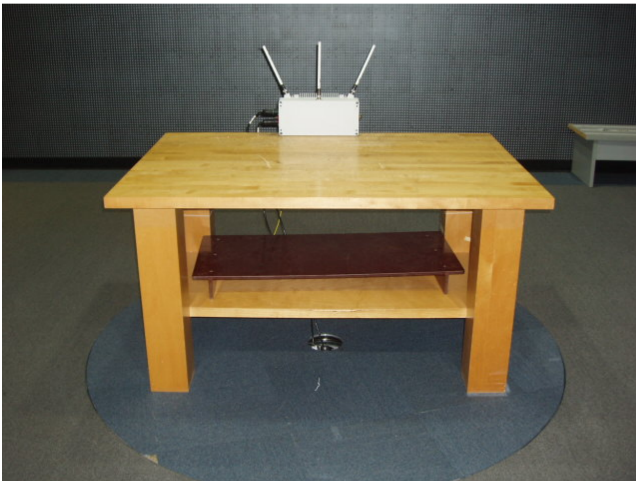
Photo 5.5-1 Radiated Emissions Test Set-up Front View
