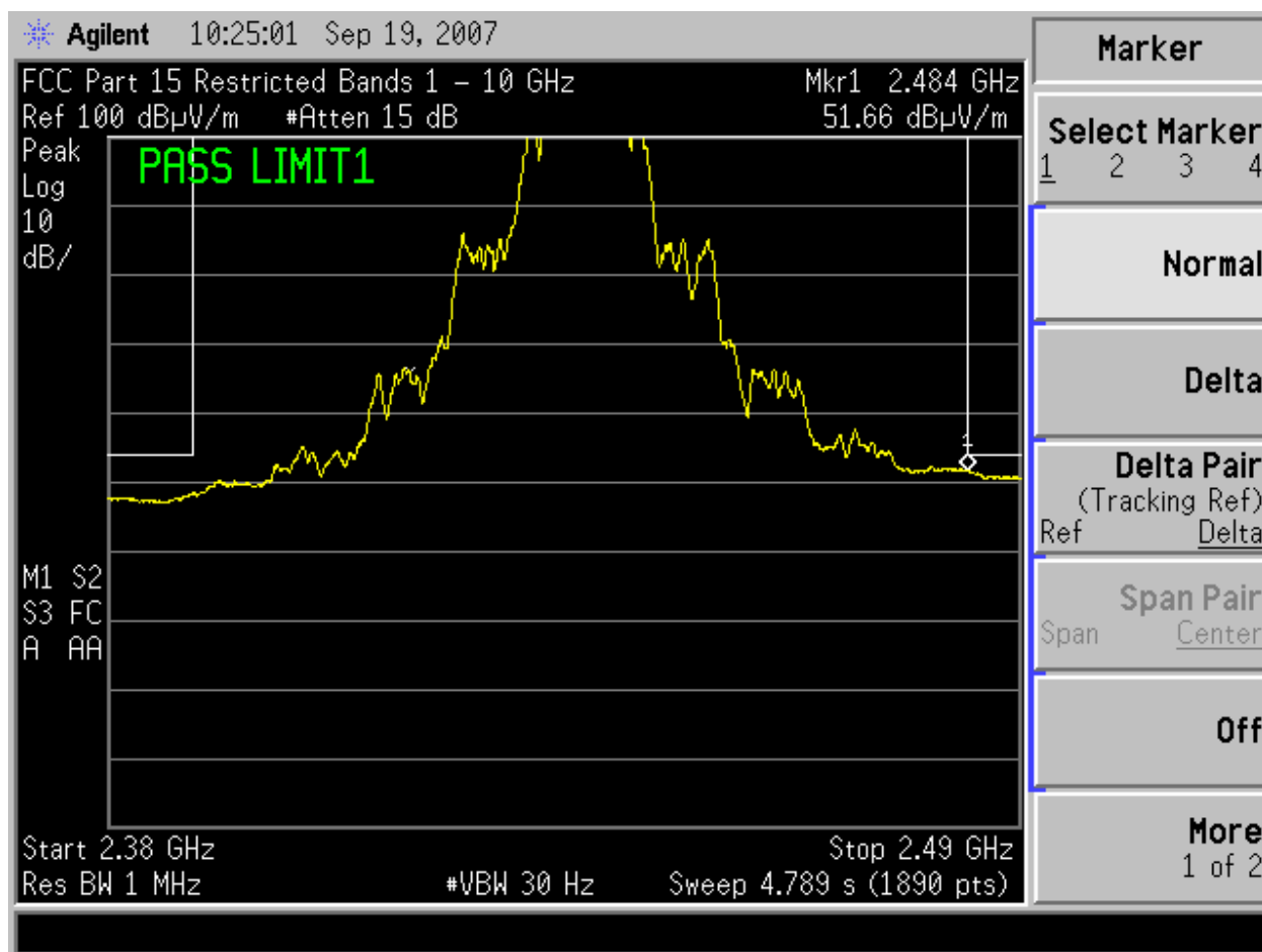
Figure 5.2-3 - FCC Class B Radiated Emissions Plot 2.38 – 2.49 GHz, Average Detector
