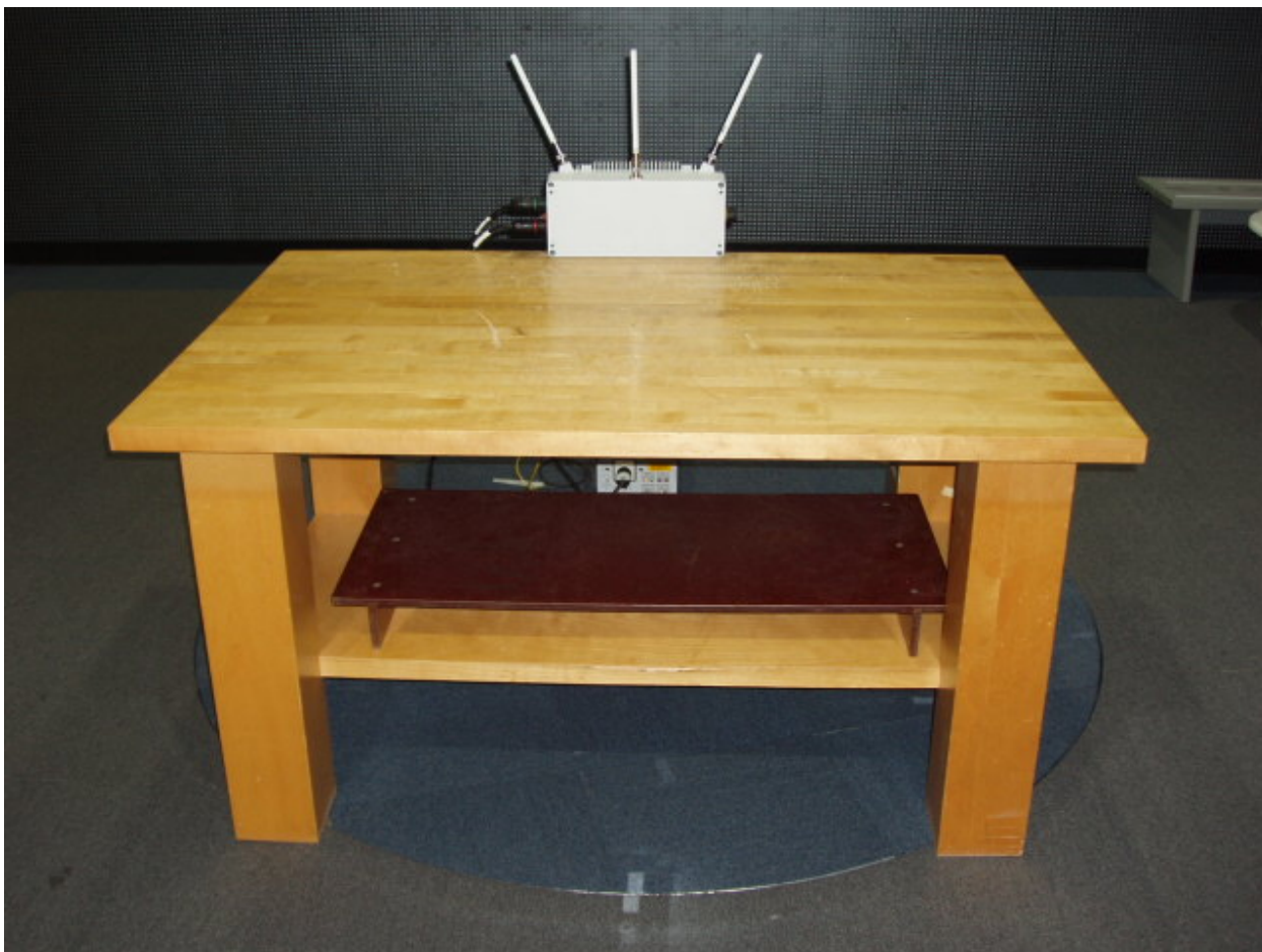
Photo 4.4-1 – Front View of Conducted Emissions Test Set-up
