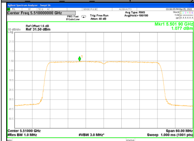
W56_11ax40_Higher_Power Spectrum Density
