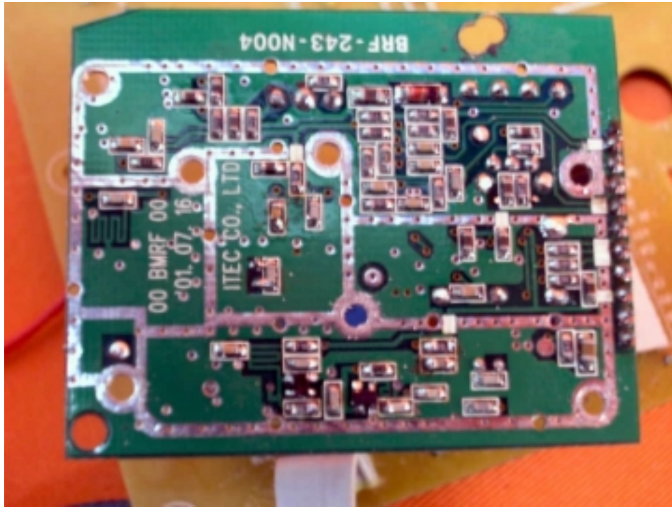
Base Oscillator PCB solder side
