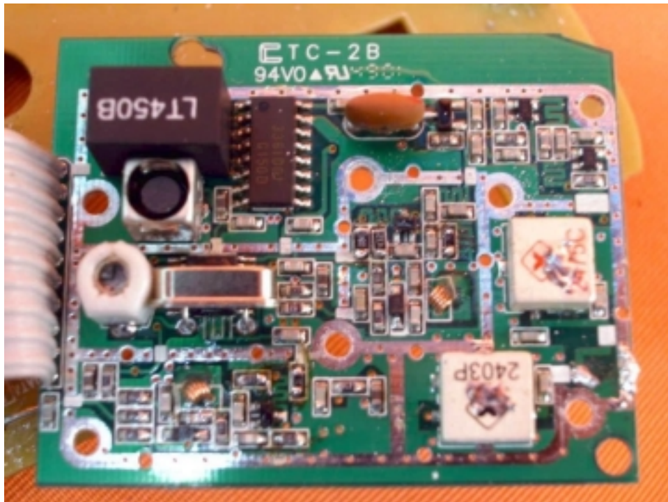
Base Oscillator PCB comp side
