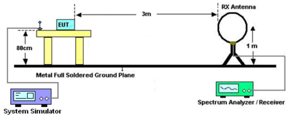
For radiated test from 30MHz to 1GHz
