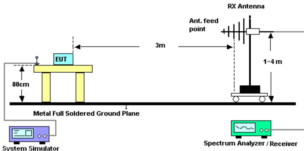
**For radiated test above 1GHz**
