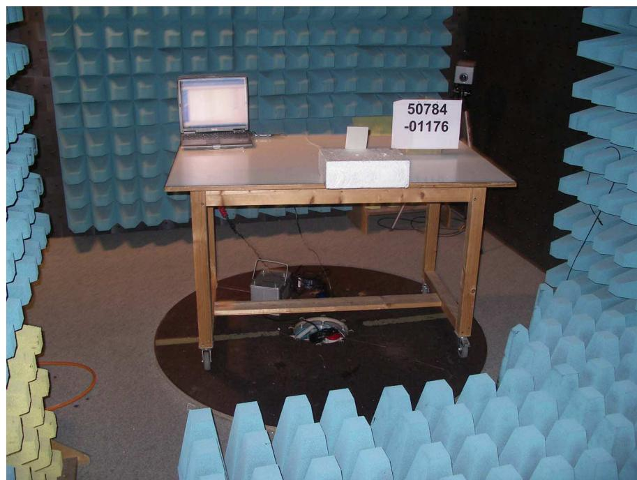
**Test setup for radiated emission measurement
