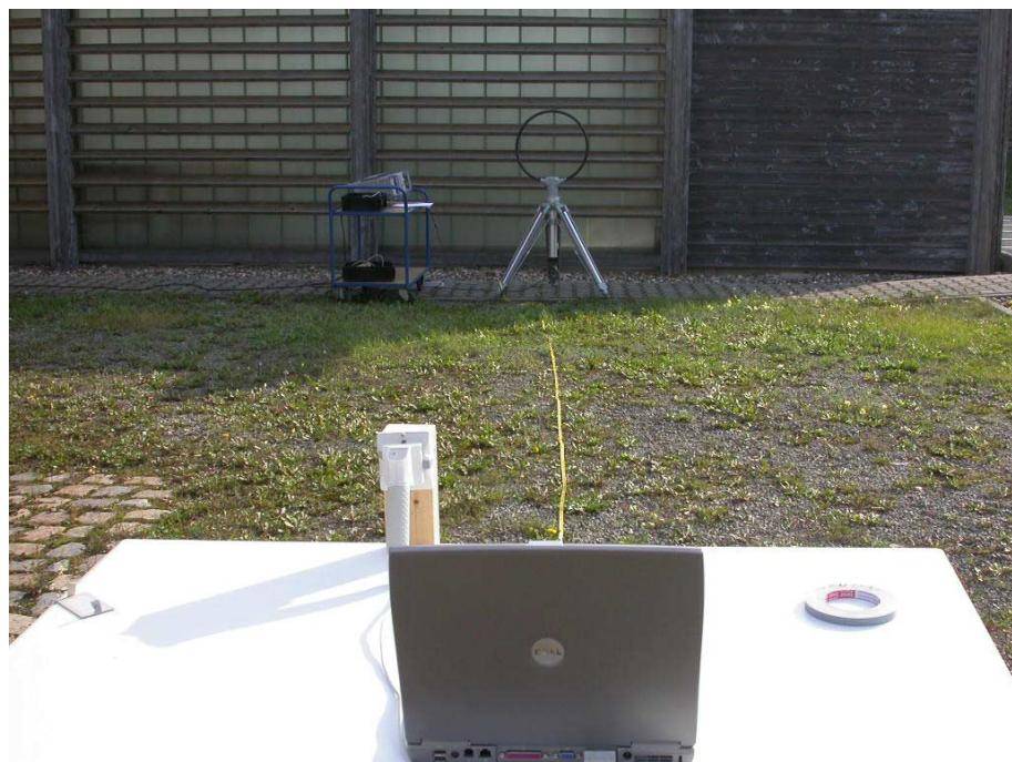
**Test setup for radiated emission measurement
