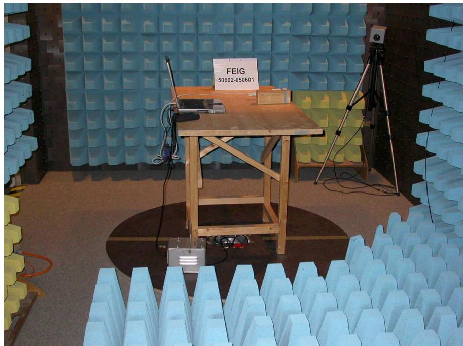
**Test setup for radiated emission measurement
