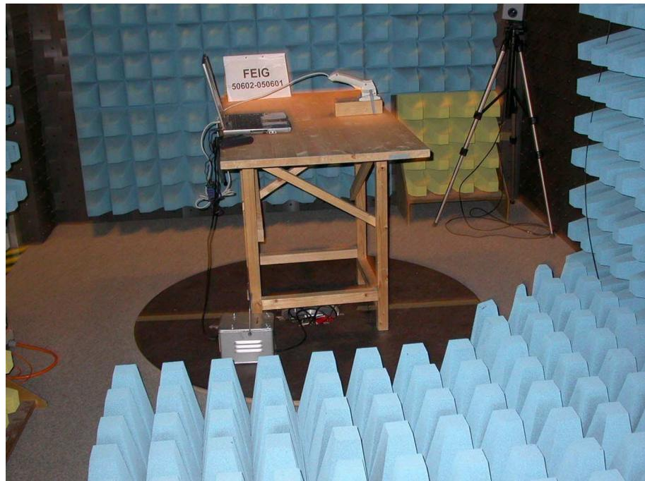
**Test setup for radiated emission measurement
