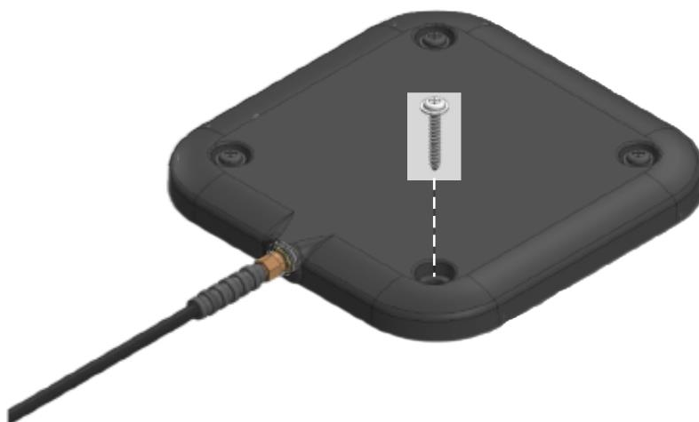
Figure 1: Drill hole + bolts (e.g. M6 x 8 mm)
