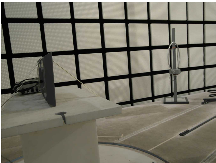
EUT with external antenna ID Ant.U580/290-FCC
