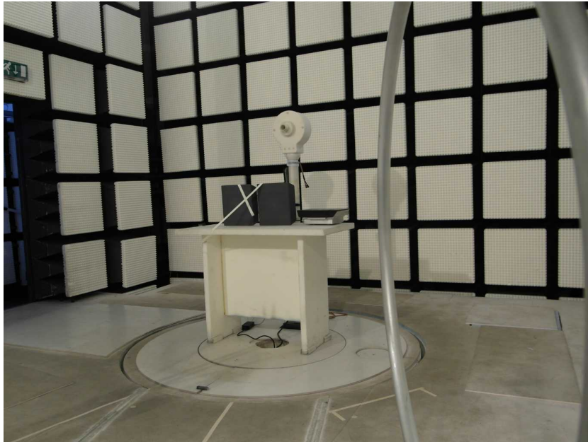
EUT with external antenna ID Ant.U580/290-FCC
