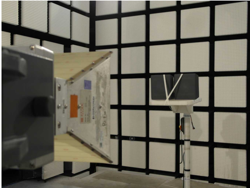
EUT with external antenna ID Ant.U580/290-FCC
