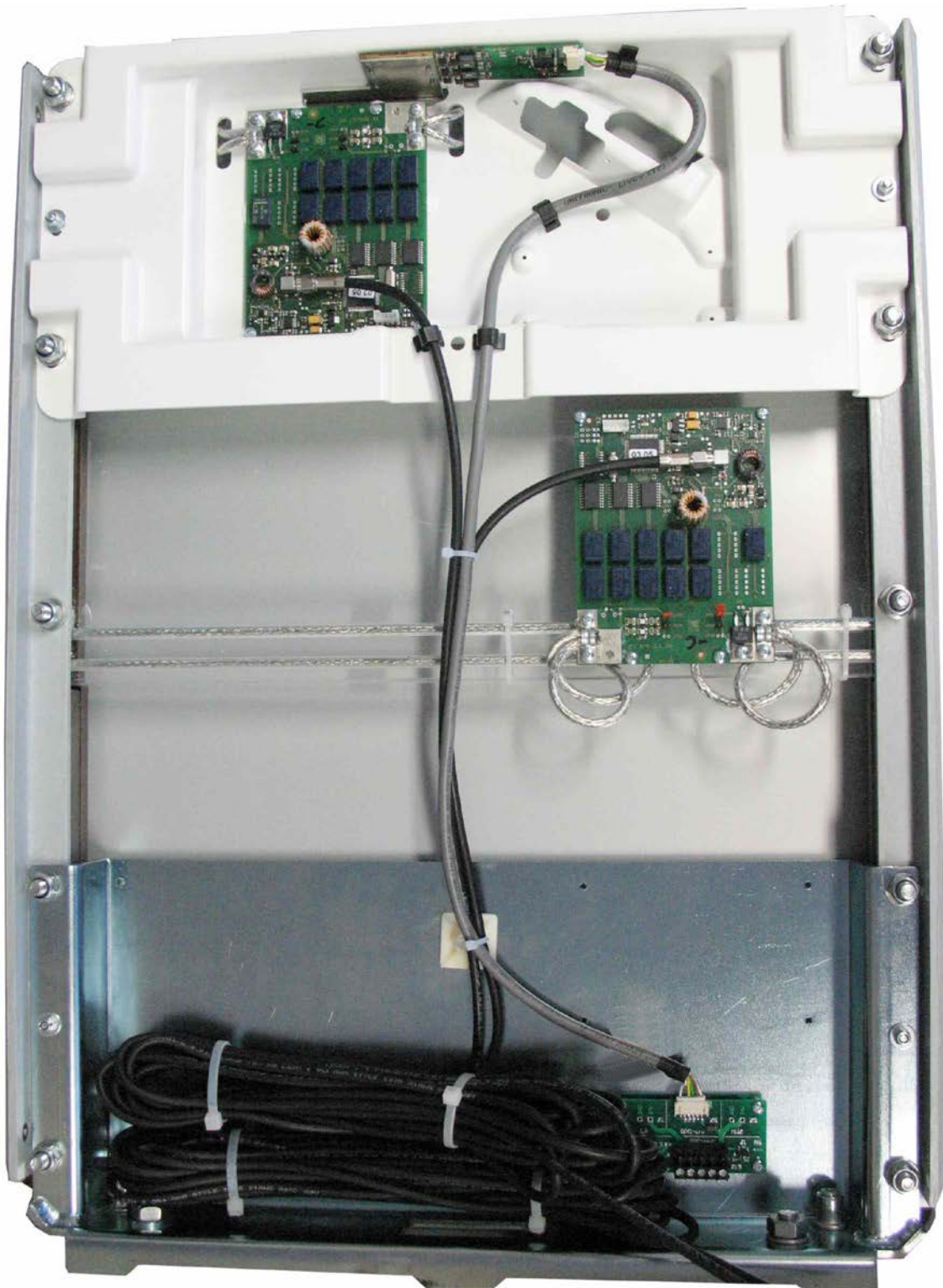
Fig. 20: Unused coaxial cables are tied in antenna Type HPDB
