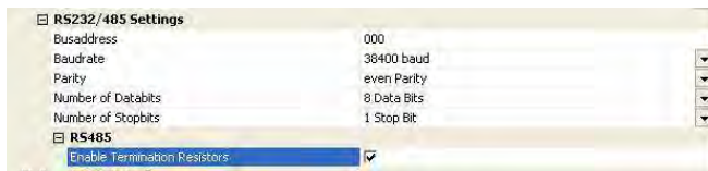
Fig. 24: Jumper settings RS485 Interface
