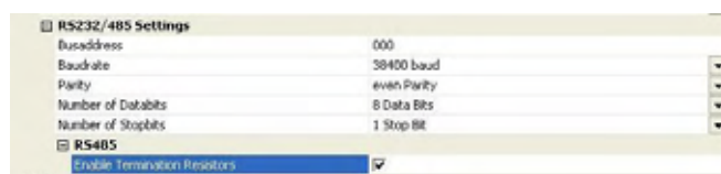
Fig. 25: Jumper settings RS485 Interface
