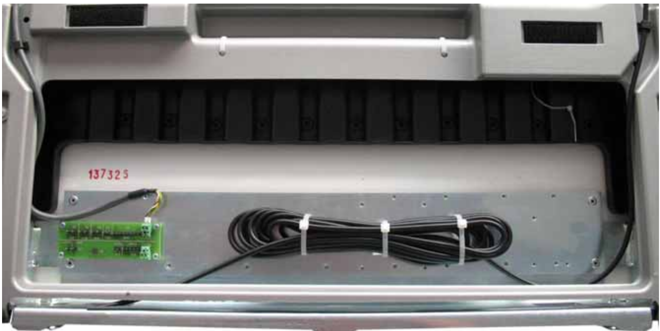
Fig. 14: Tie together the cables in an antenna Type B
