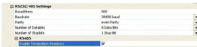
Fig. 25: Jumper settings RS485 Interface
