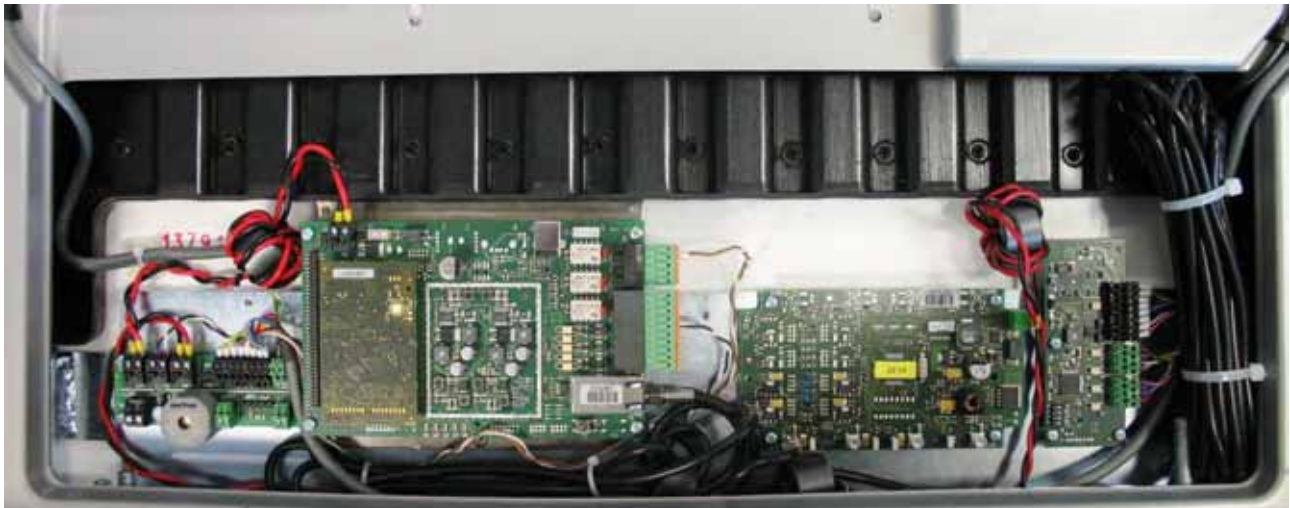
Fig. 13: Connection of the components in an antenna Type A
