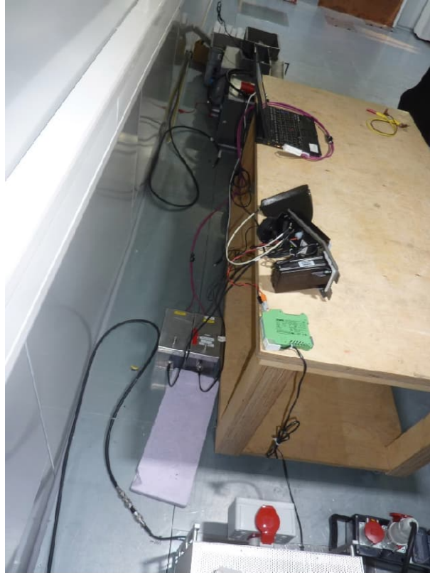
Test setup shielded chamber M155 AC powerline conducted emissions
